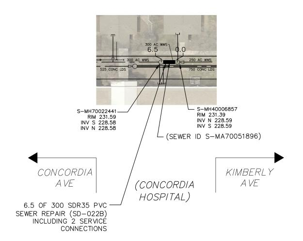
SEWER JUNCTION INFORMATION FROM SEWER VIDEO INSPECTION SEWER ID S-MA70051896 DISTANCE FROM MH ID S-MH40006857 DISTANCE DIAMETER CLOCK 1.1 150 5.0 10
