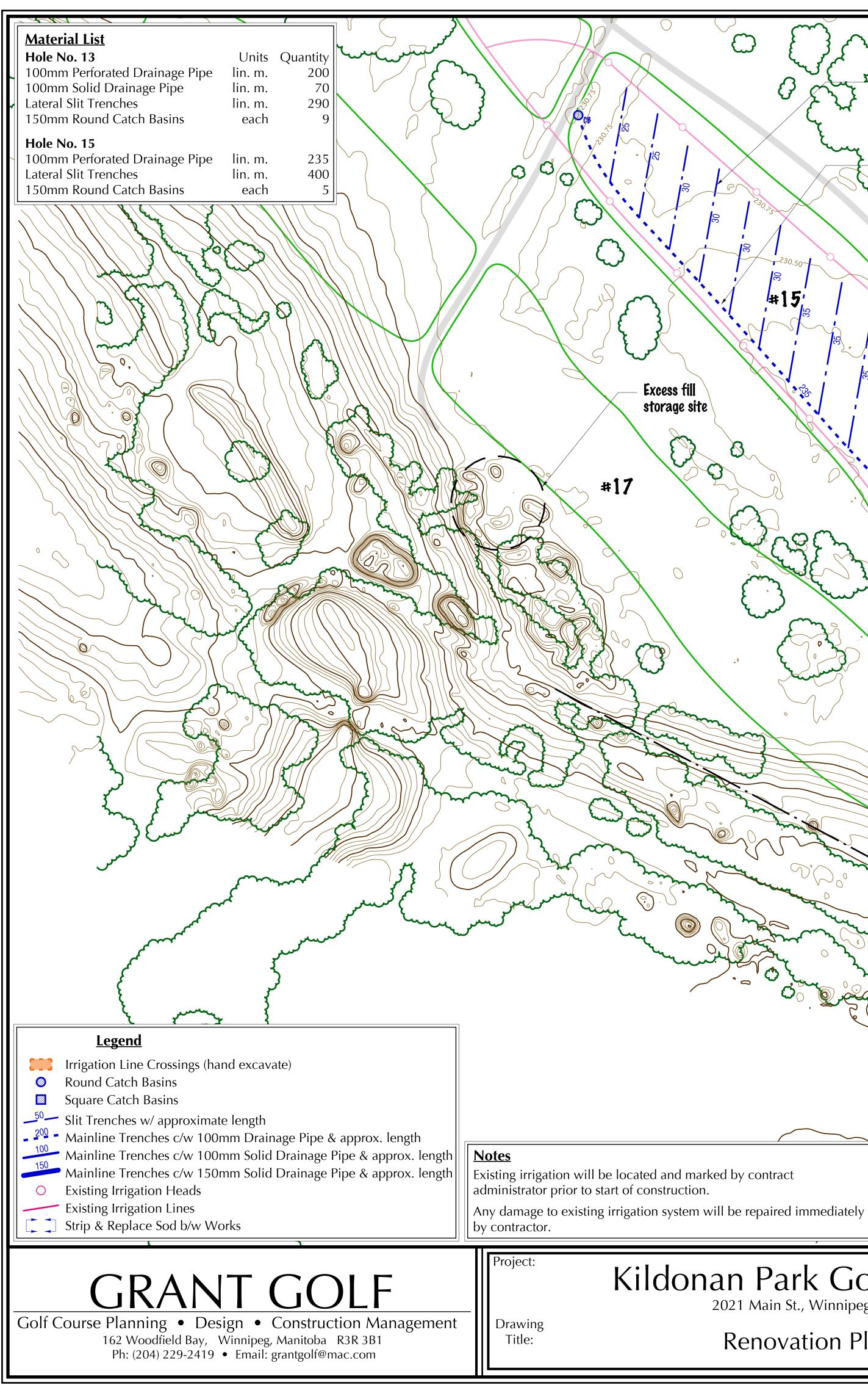
Trench lateral slit drains at approx. 10 metre intervals, starting & end grades (inverts) to be marked on-site by contract administrator (see details 6/L4 & 7/L4), haul fill to storage site on east side of #17 fairway
