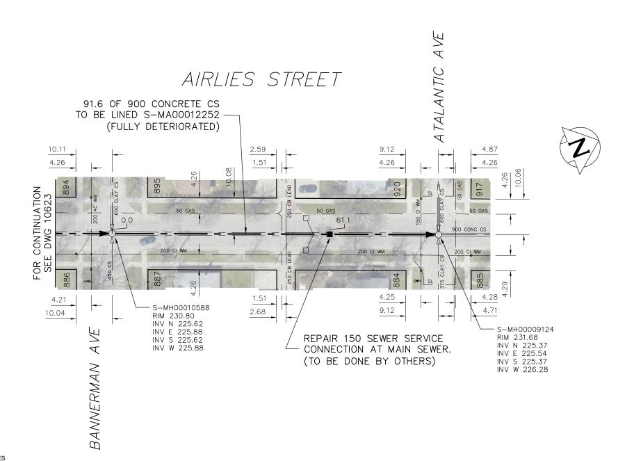
SEWER JUNCTION INFORMATION FROM SEWER VIDEO INSPECTION SEWER ID S-MA00012252 DISTANCE FROM MH ID S-MH00010588 DISTANCE DIAMETER CLOCK 22.4 150 22.4 11 30.0 150 30.0 150 37.2 150 43.4 150 12 45.0 150 45.0 150 11 47.4 150 10 47.9 150 150 55.4 10 56.7 150 66.0 150 73.8 150 150 81.9 11
