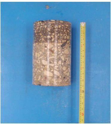
Core sample from Testhole TH05
