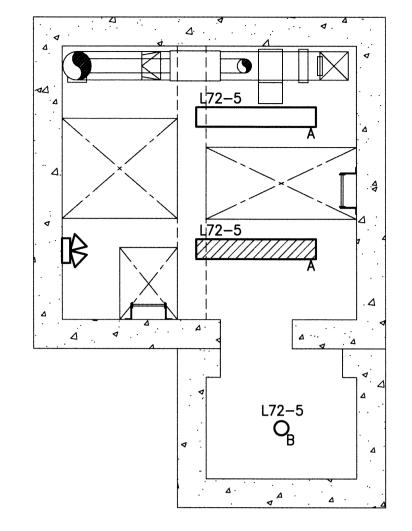
ELECTRICAL ROOM FLOOR PLAN SCALE: 1:40
