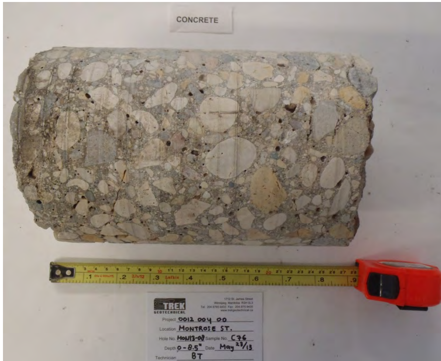
Photo 8: Concrete Core Sample from Test Hole MON13-08
