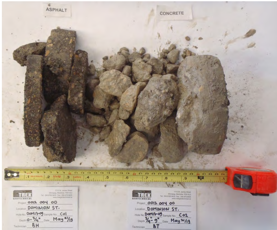
Photo 9: Asphalt and Concrete Core Sample from Test Hole DOM13-09
