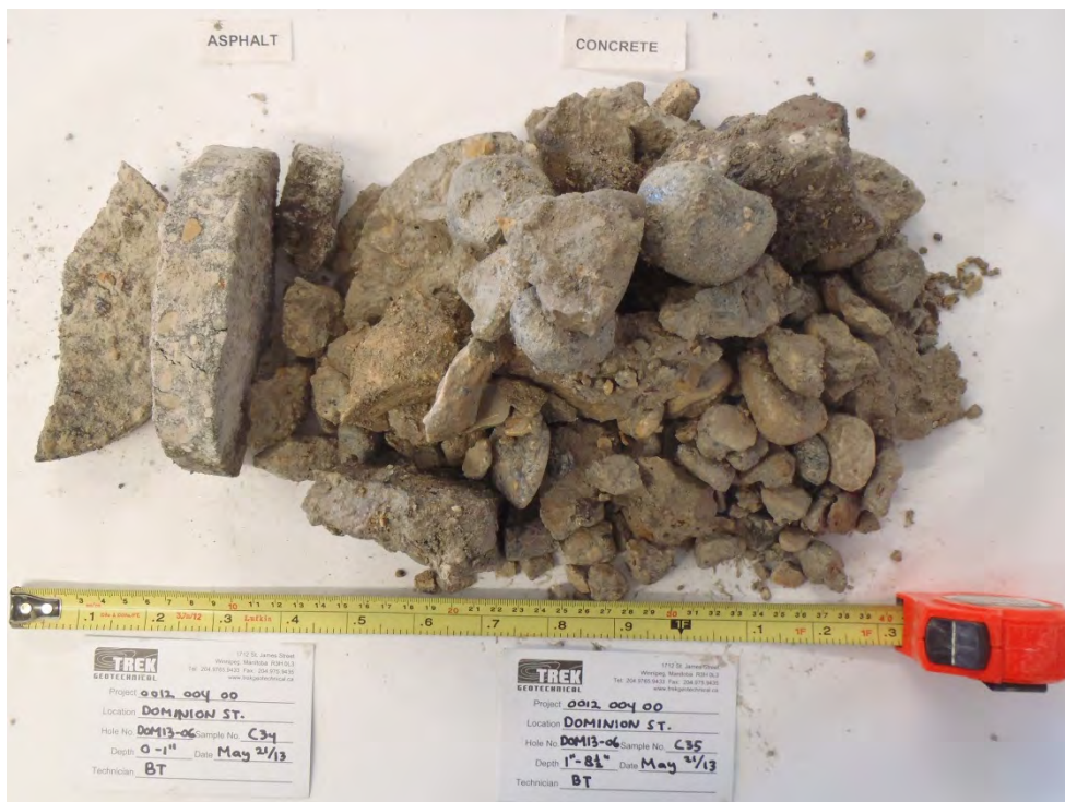
Photo 6: Asphalt and Concrete Core Sample from Test Hole DOM13-06
