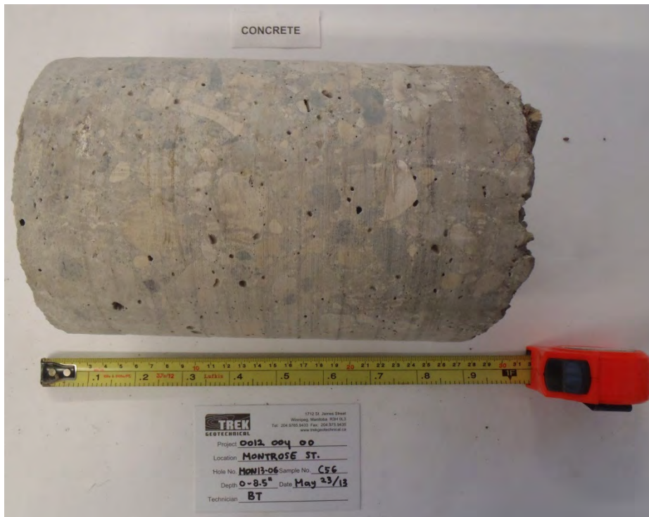
Photo 6: Concrete Core Sample from Test Hole MON13-06
