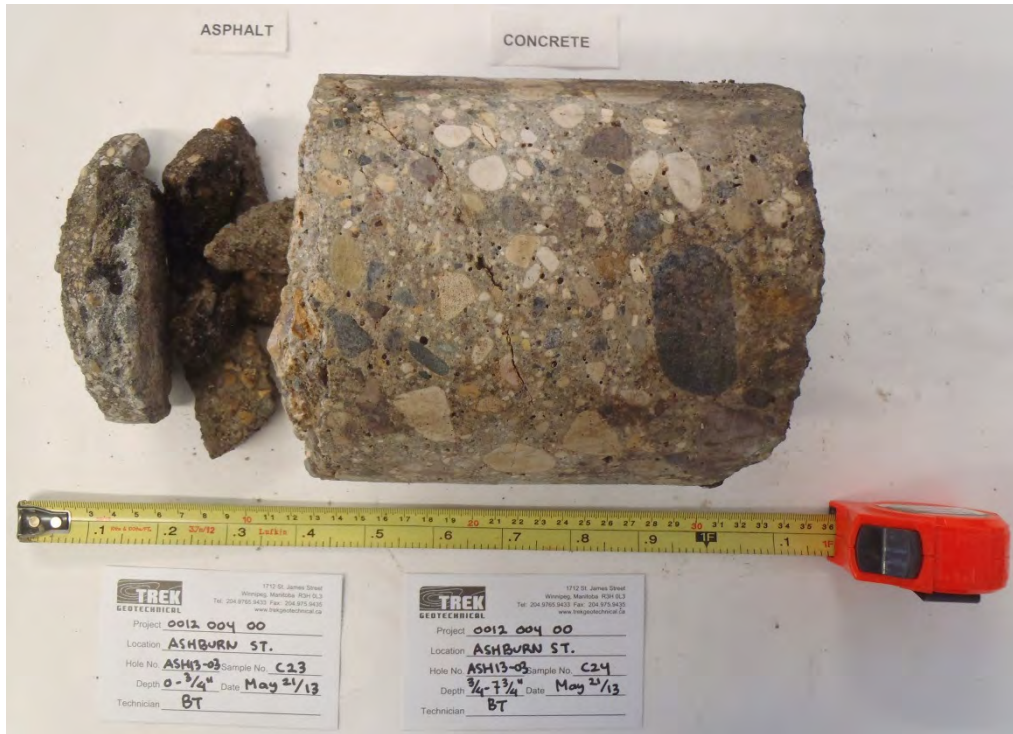
Photo 3: Asphalt and Concrete Core sample from Test Hole ASH13-03
