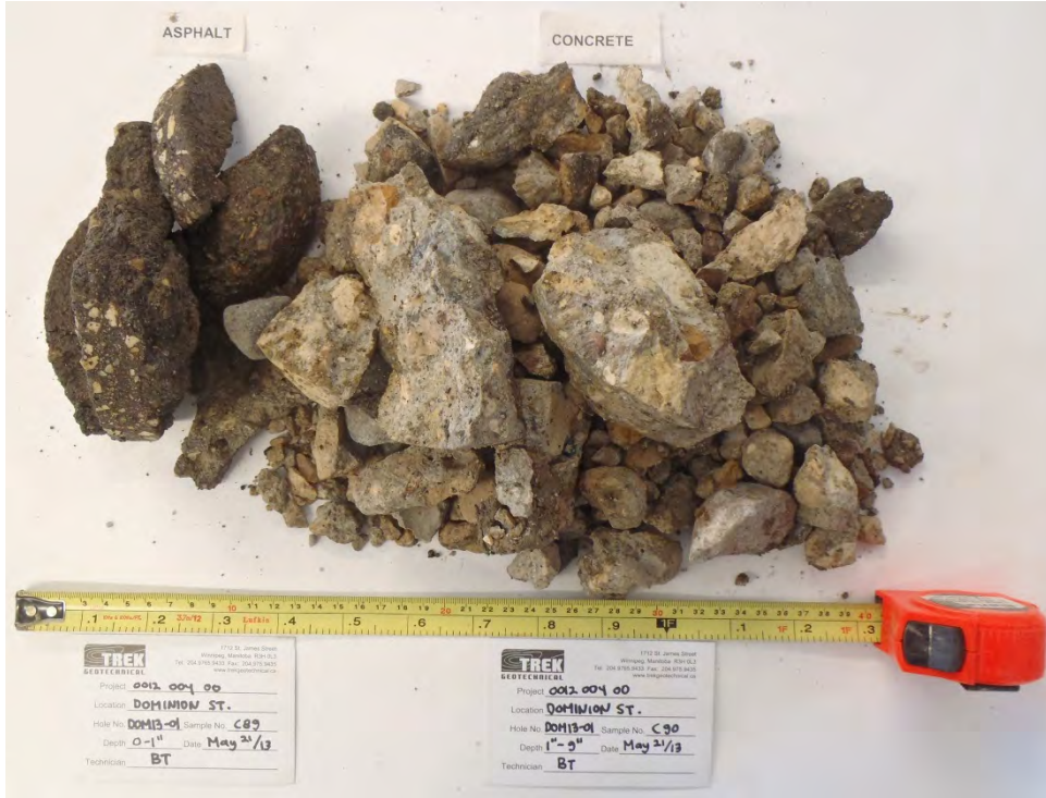
Photo 1: Asphalt and Concrete Core Sample from Test Hole DOM13-01
