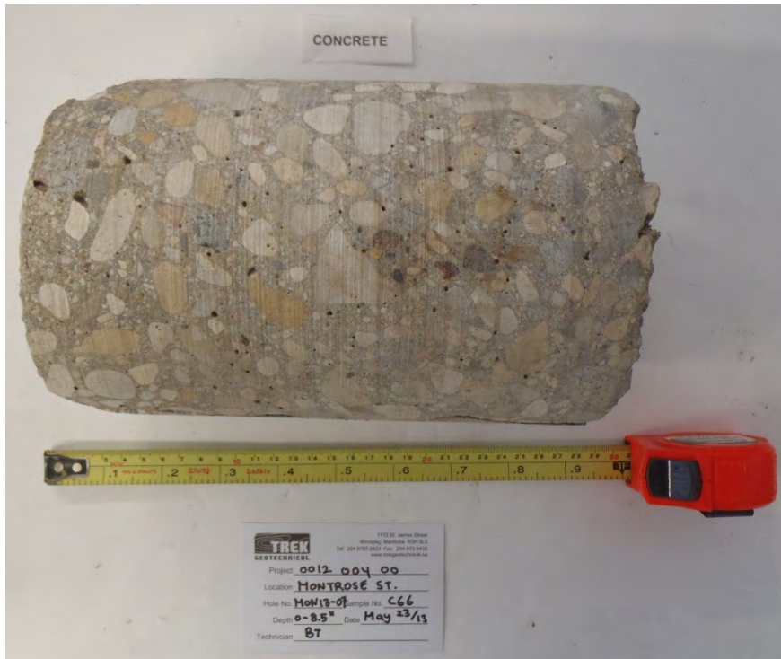
Photo 7: Concrete Core Sample from Test Hole MON13-07
