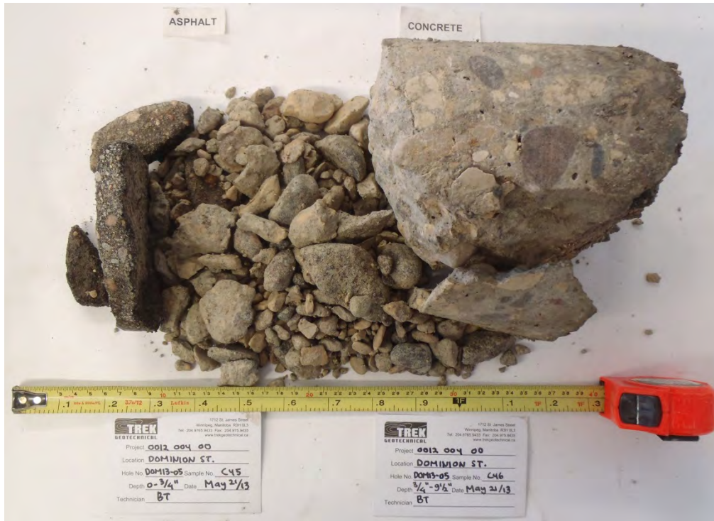
Photo 5: Asphalt and Concrete Core Sample from Test Hole DOM13-05
