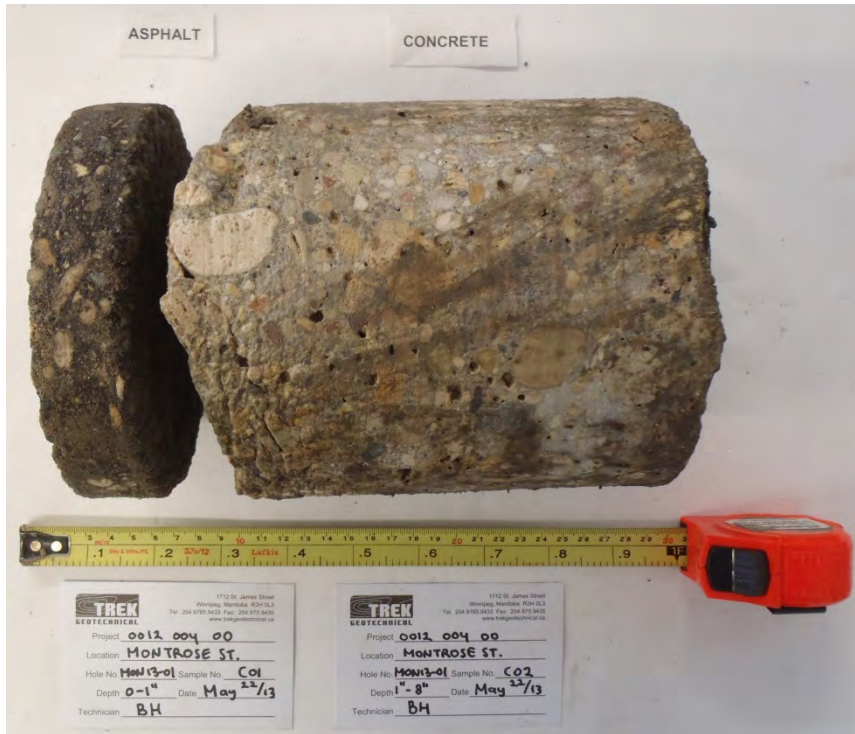
Photo 1: Asphalt and Concrete Core Sample from Test Hole MON13-01
