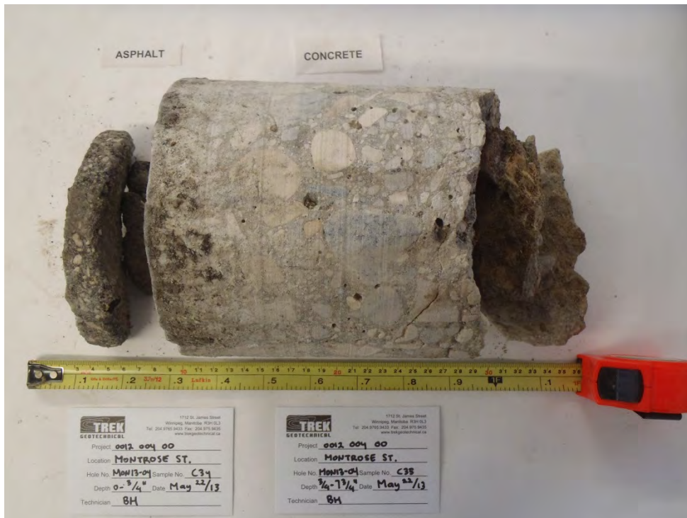
Photo 4: Asphalt and Concrete Core Sample from Test Hole MON13-04
