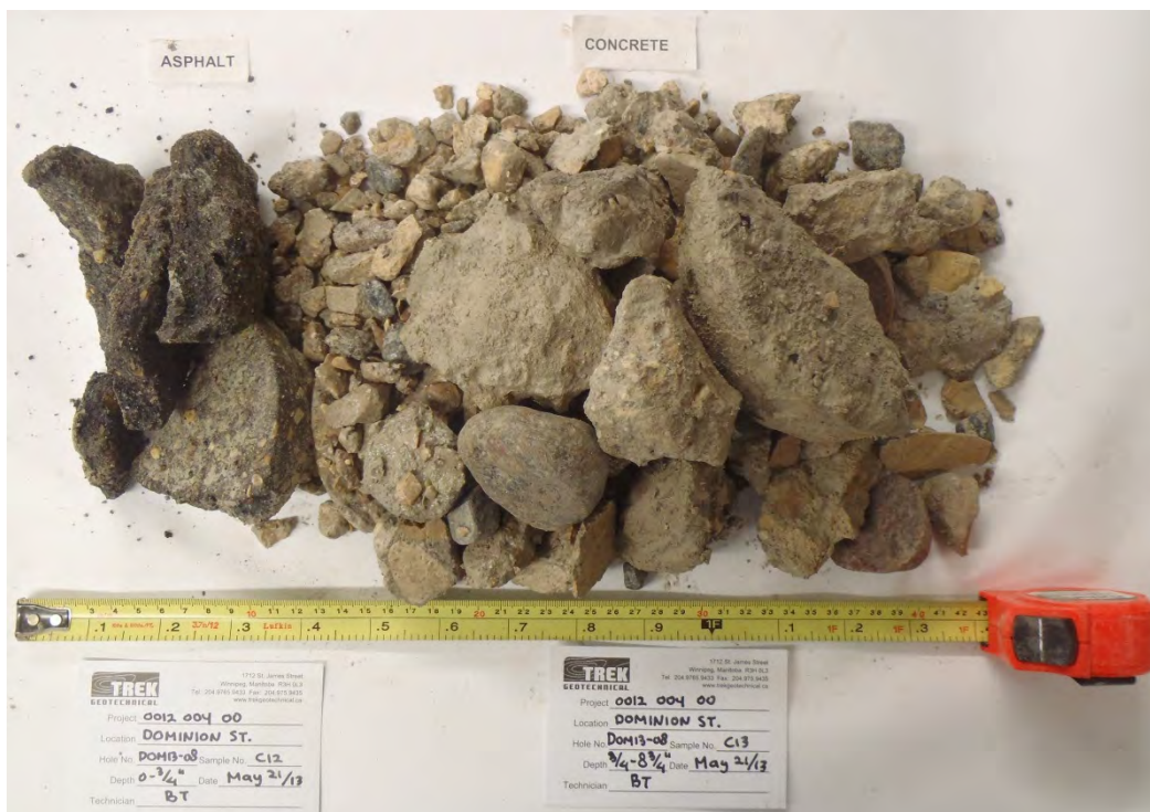
Photo 8: Asphalt and Concrete Core Sample from Test Hole DOM13-08
