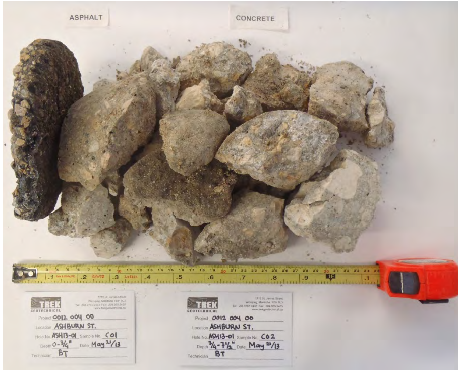
Photo 1: Asphalt and Concrete Core Sample from Test Hole ASH13-01
