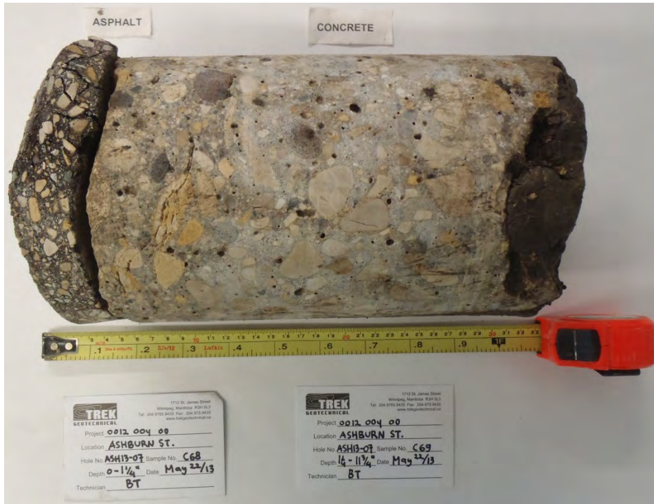
Photo 7: Asphalt and Concrete core sample from Test Hole ASH13-07
