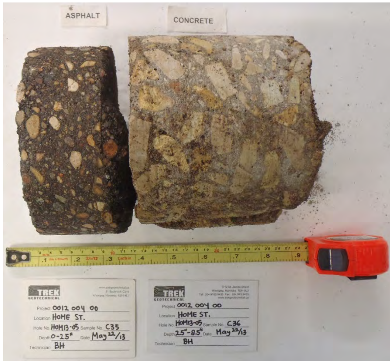
Photo 5: Asphalt and Concrete Core Sample from Test Hole HOM13-05
