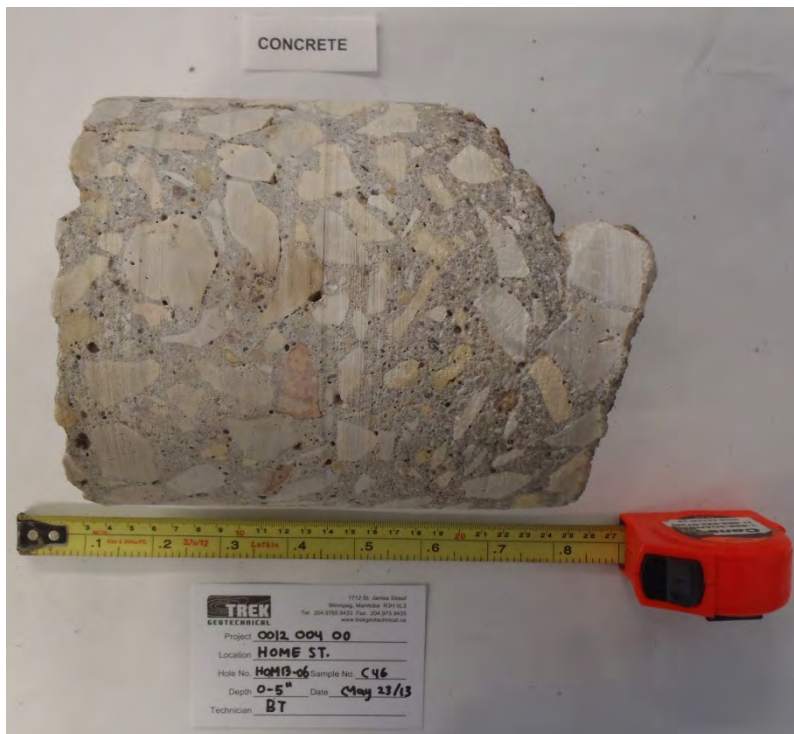
Photo 6: Concrete Core Sample from Test Hole HOM13-06
