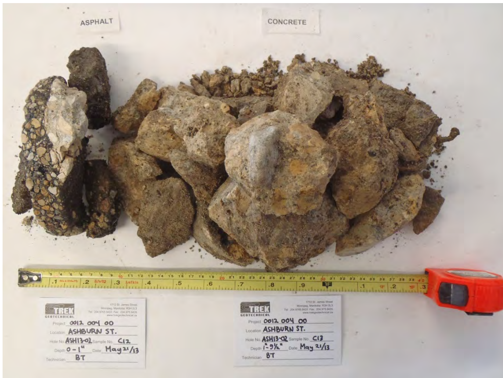
Photo 2: Asphalt and Concrete Core Sample from Test Hole ASH13-02
