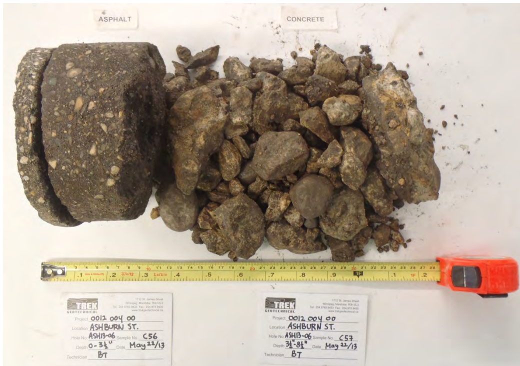
Photo 6: Asphalt and Concrete Core sample from Test Hole ASH13-06
