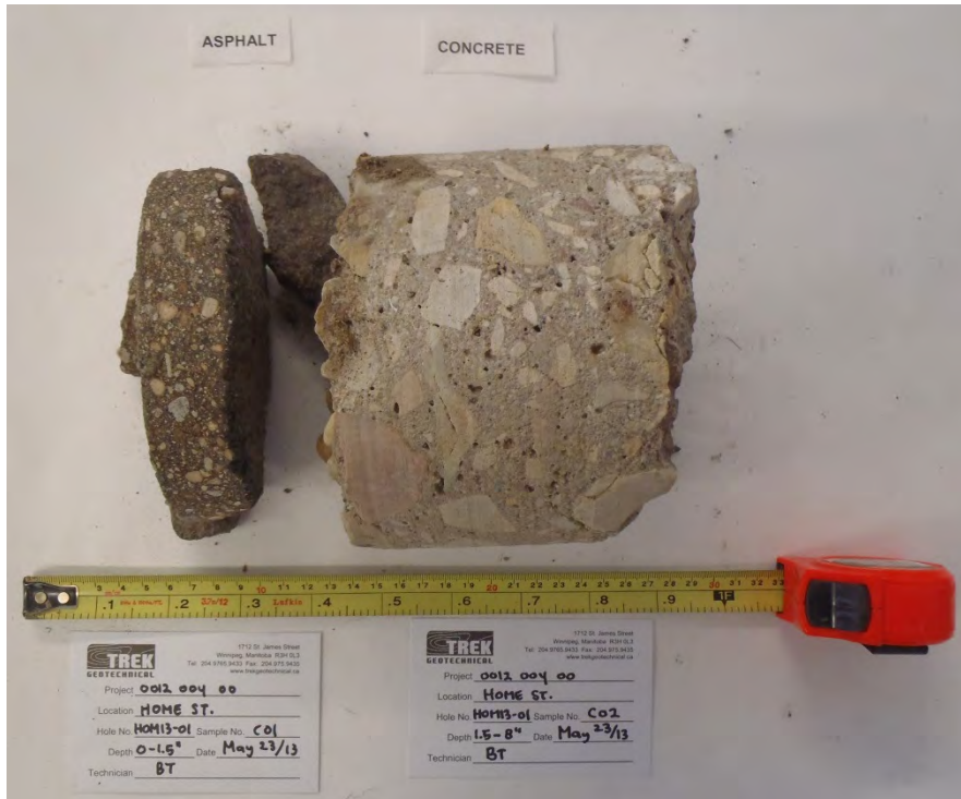
Photo 1: Asphalt and Concrete Core Sample from Test Hole HOM13-01
