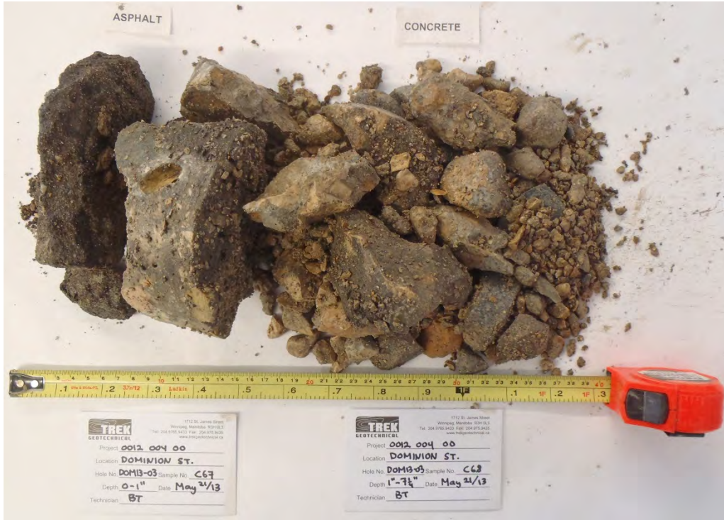
Photo 3: Asphalt and Concrete Core Sample from Test Hole DOM13-03
