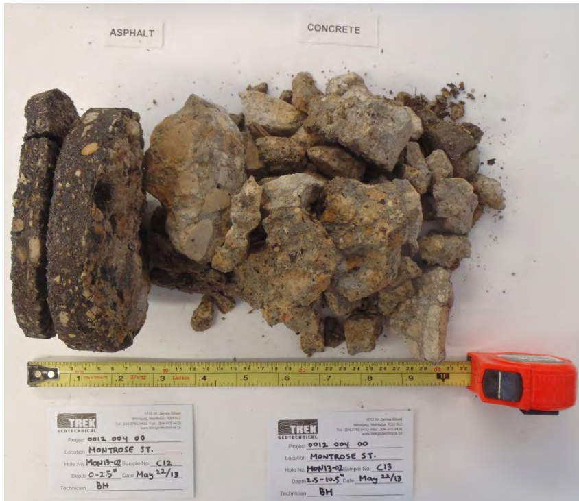
Photo 2: Asphalt and Concrete Core Sample from Test Hole MON13-02
