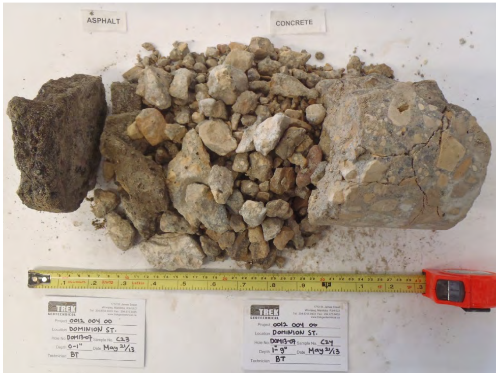
Photo 7: Asphalt and Concrete Core Sample from Test Hole DOM13-07
