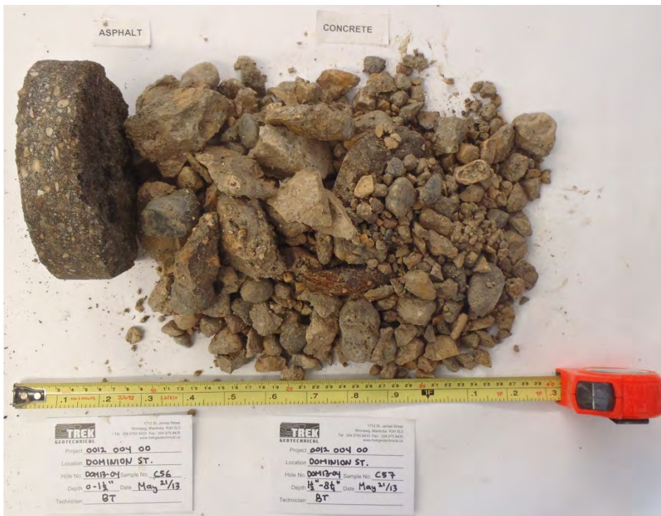
Photo 4: Asphalt and Concrete Core Sample from Test Hole DOM13-04
