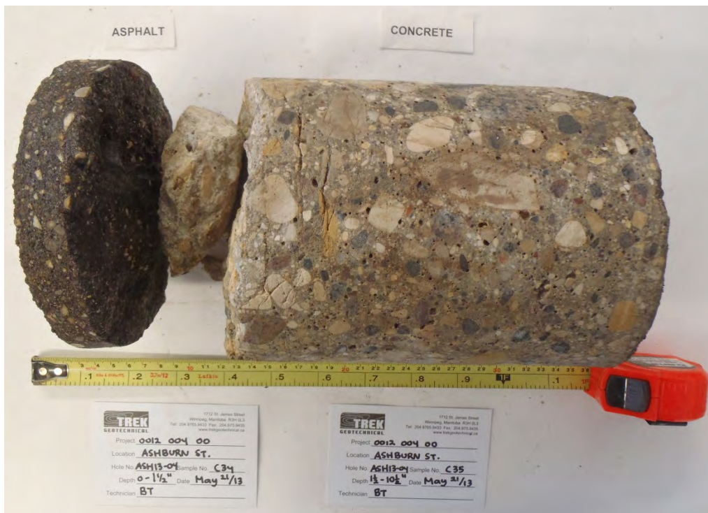
Photo 4: Asphalt and Concrete Core sample from Test Hole ASH13-04
