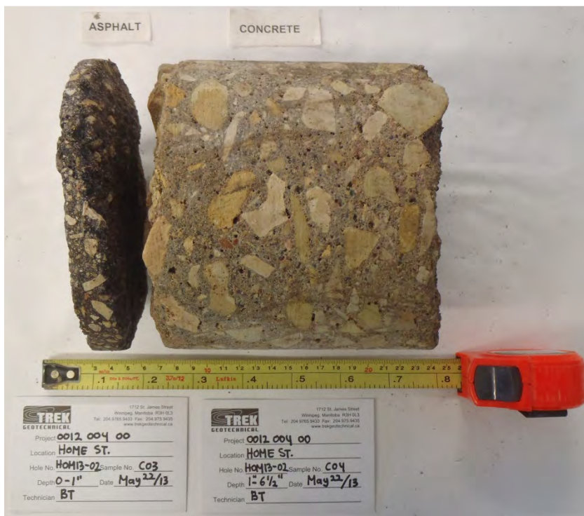
Photo 2: Asphalt and Concrete Core Sample from Test Hole HOM13-02
