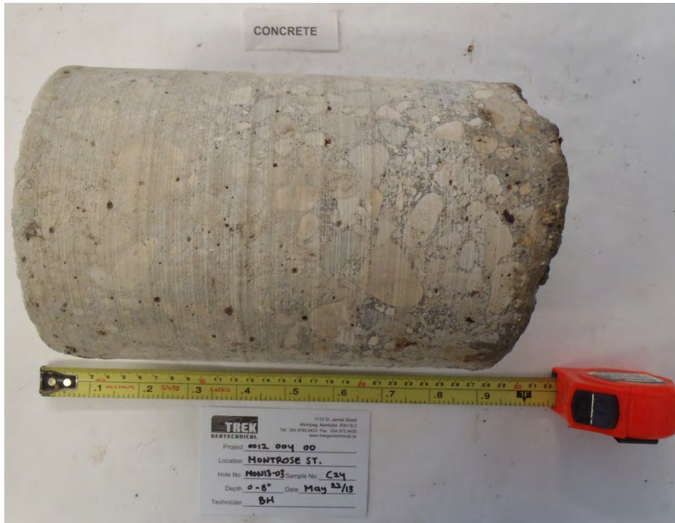
Photo 3: Concrete Core Sample from Test Hole MON13-03
