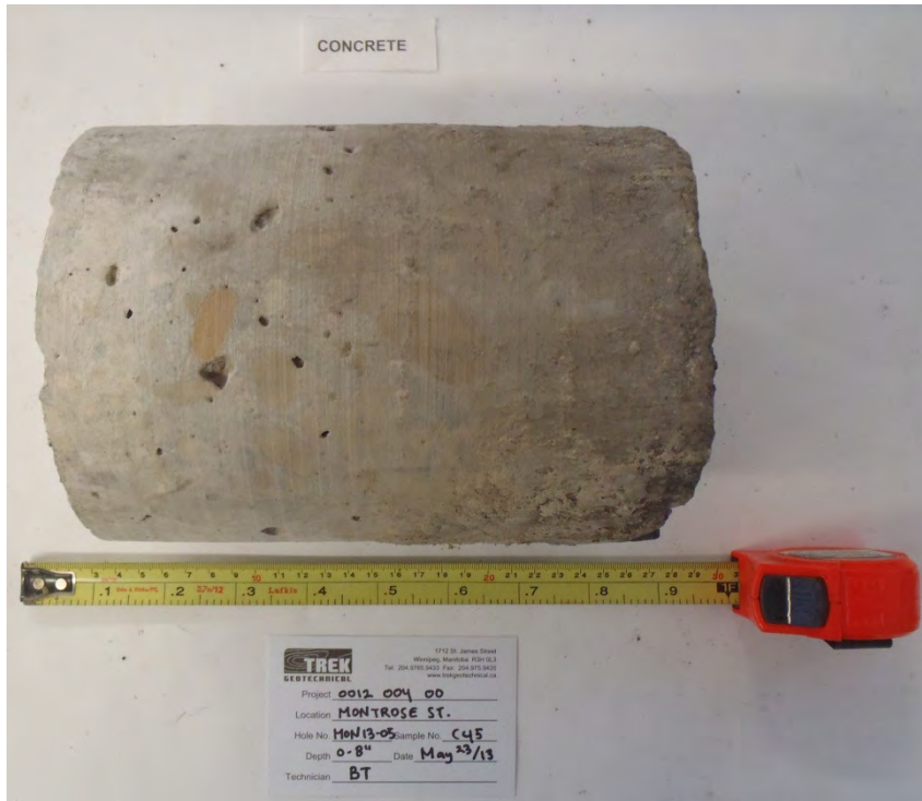
Photo 5: Concrete Core Sample from Test Hole MON13-05
