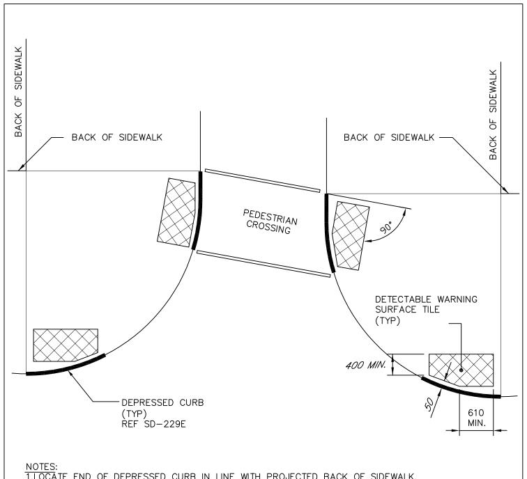
1.LOCATE END OF DEPRESSED CURB IN LINE WITH PROJECTED BACK OF SIDEWALK. 2.CONSTRUCT FLARES IN ACCORDANCE WITH SD-229A
