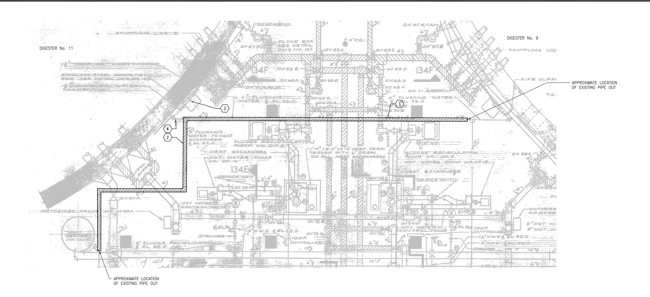
1 DEMOLISH AND REMOVE PREVIOUSLY ABANDONED 100Ø FLUSHING WATER PIPE.
