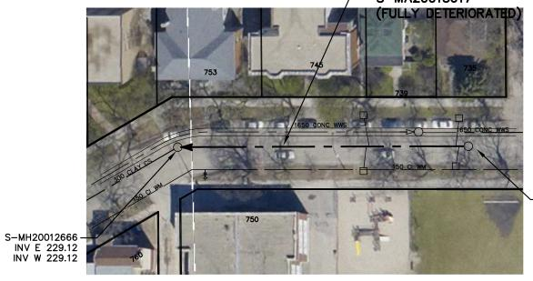
SEWER JUNCTION INFORMATION FROM SEWER VIDEO INSPECTION SEWER ID S-MA20013617 DISTANCE FROM MH ID S-MH20012337 DISTANCE DIAMETER 2.0 150 10 2.7 150 16.0 150 150 25.3 10 150 25.9 3 150 38.7 3 54.1 150 3 57.2 150 10
