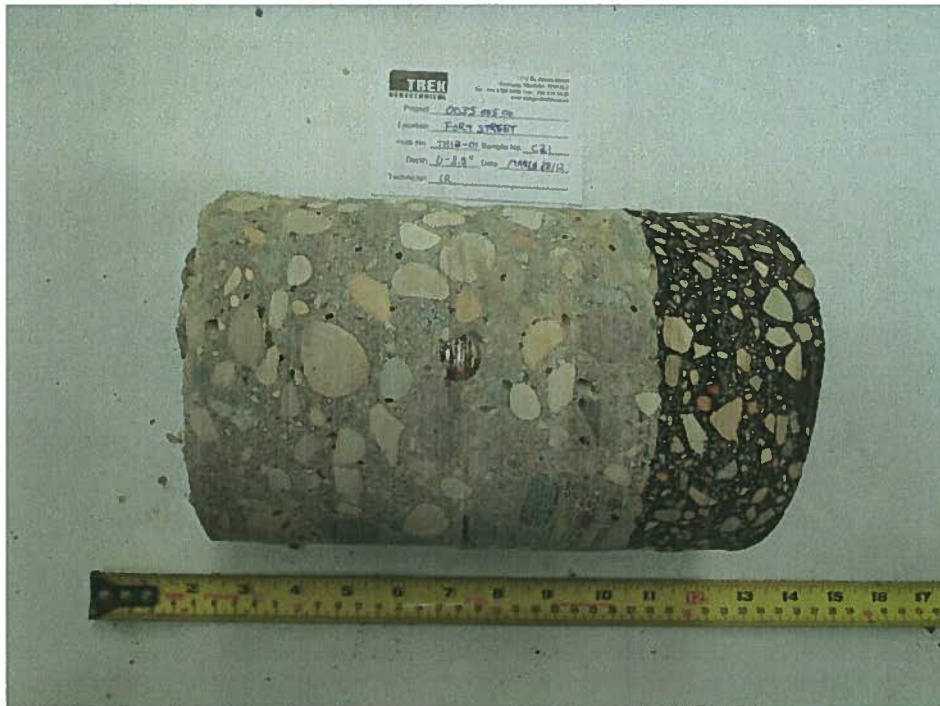
Photo 1: Asphalt and concrete core sample from Test Hole TH12-01
