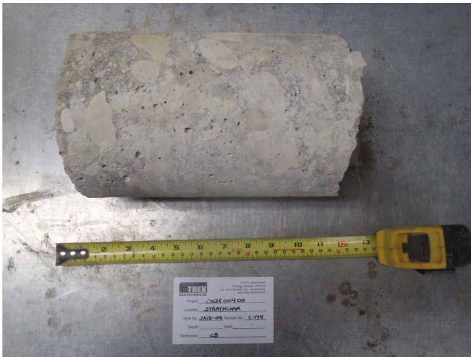
Photo 21: Concrete core sample from Test Hole SA12-04
