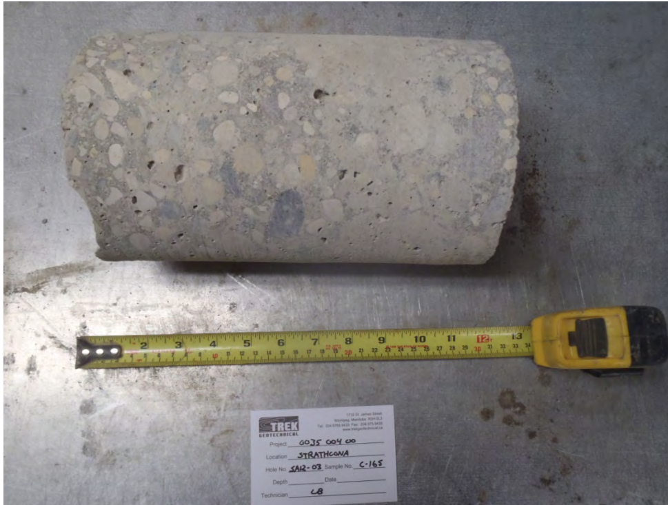
Photo 20: Concrete core sample from Test Hole SA12-03
