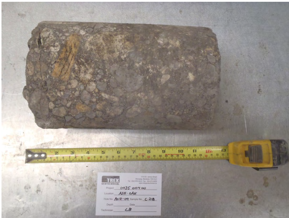
Photo 29: Concrete core sample from Test Hole AO12-04
