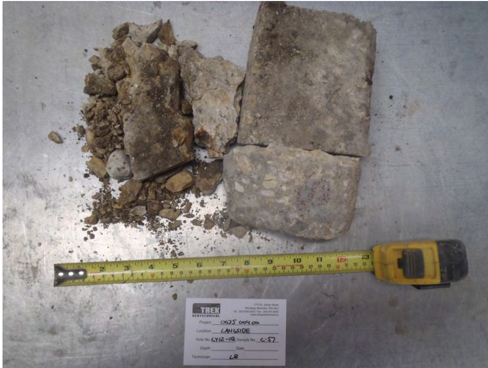
Photo 8: Concrete core sample from Test Hole LY12-02
