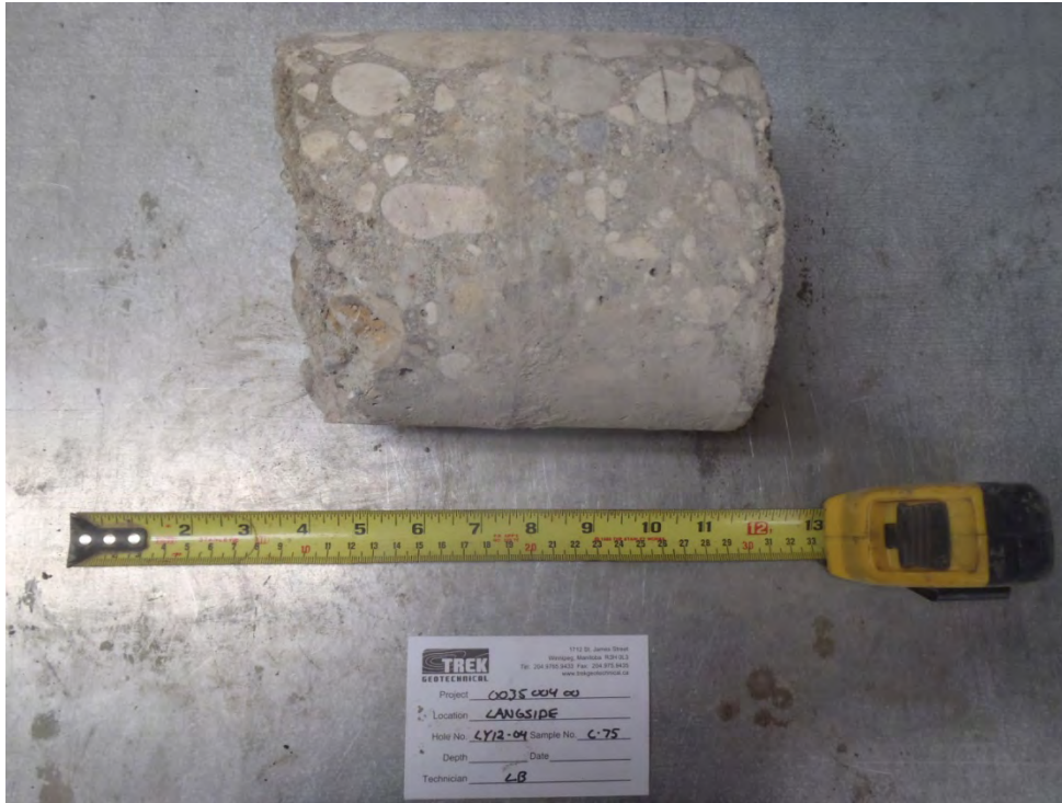
Photo 10: Concrete core sample from Test Hole LY12-04
