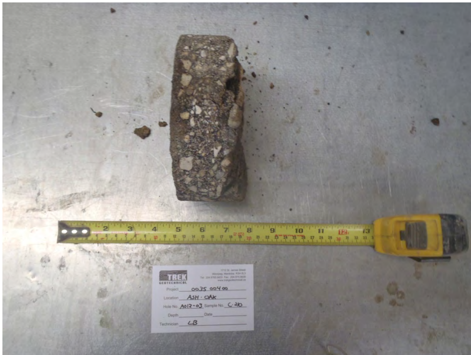
Photo 27: Asphalt core sample from Test Hole AO12-03
