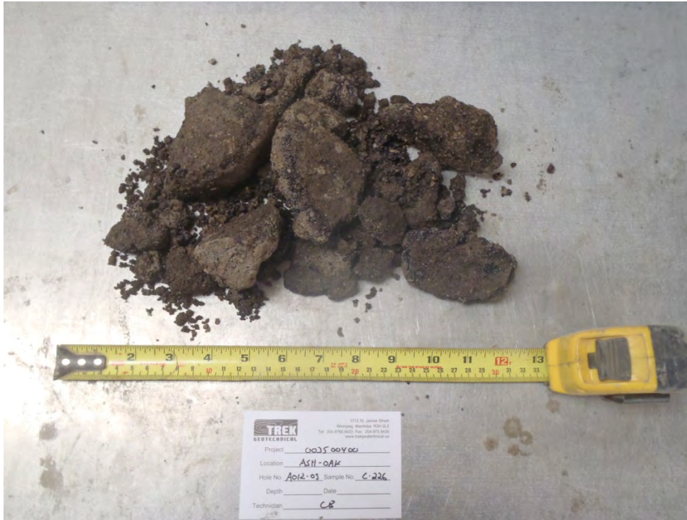
Photo 30: Asphalt core sample from Test Hole AO12-05
