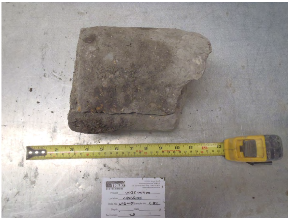
Photo 11: Concrete core sample from Test Hole LY12-05
