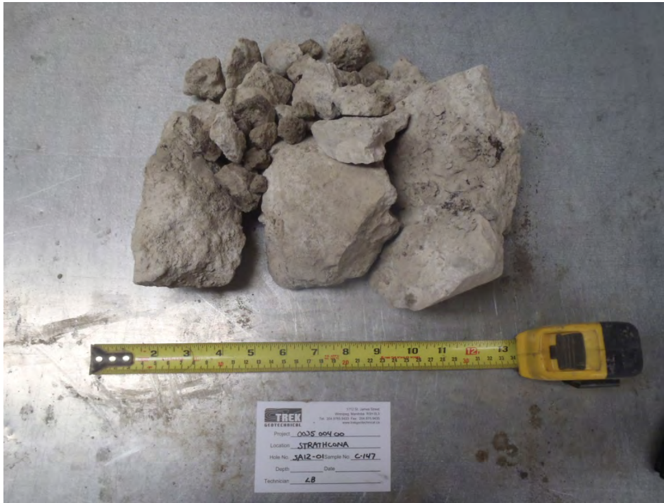
Photo 18: Concrete core sample from Test Hole SA12-01
