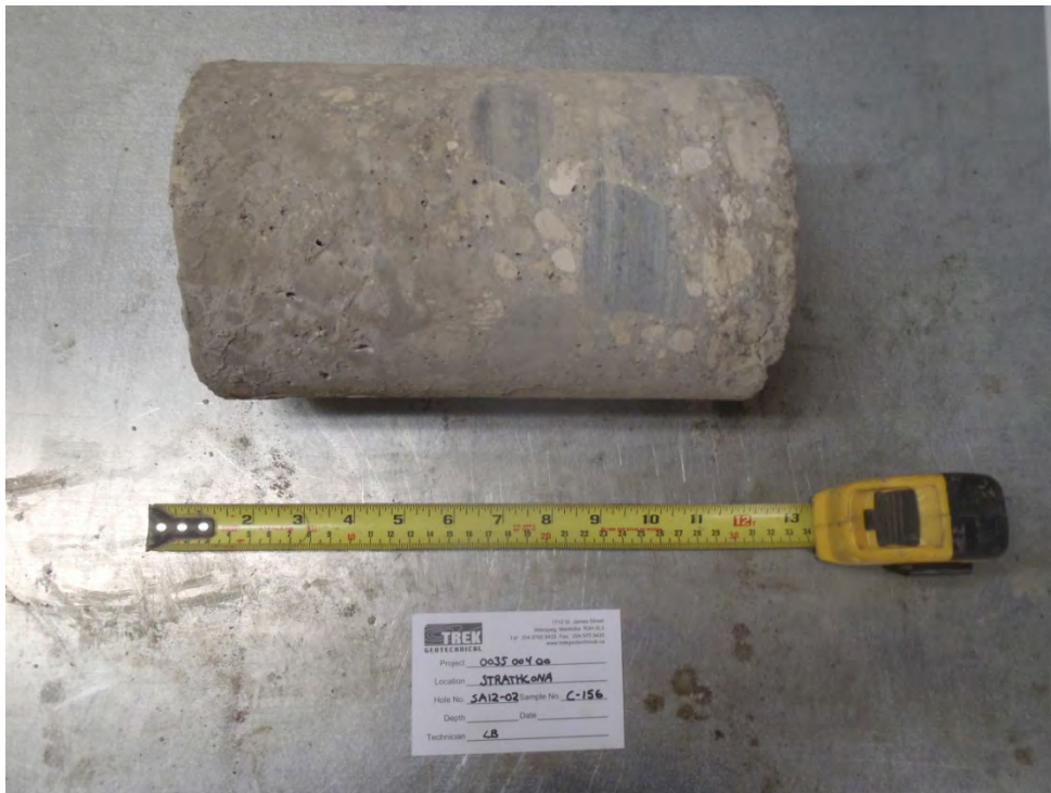
Photo 19: Concrete core sample from Test Hole SA12-02
