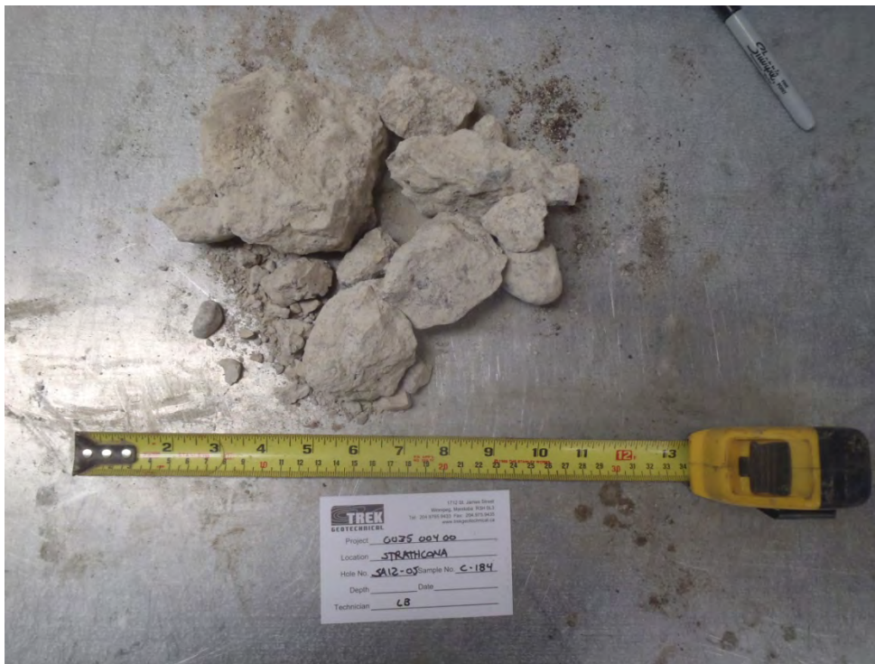
Photo 23: Concrete core sample from Test Hole SA12-05
