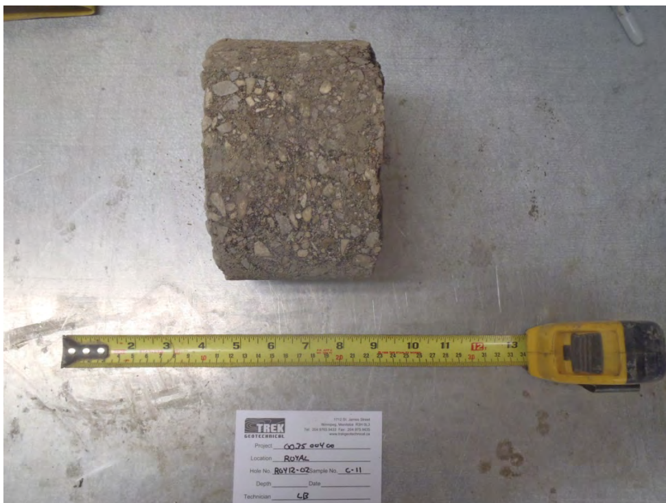
Photo 2: Asphalt core sample from Test Hole ROY12-02
