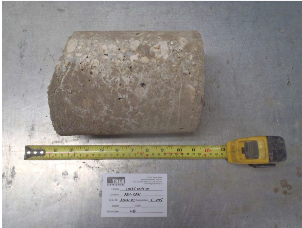
Photo 34: Concrete core sample from Test Hole AO12-07
