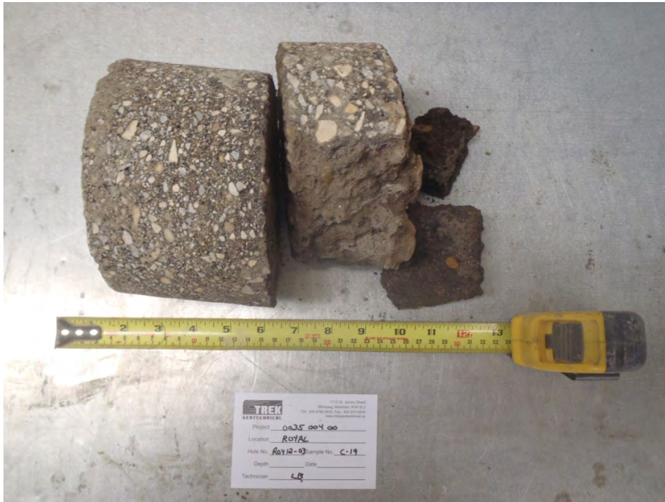
Photo 3: Asphalt core sample from Test Hole ROY12-03
