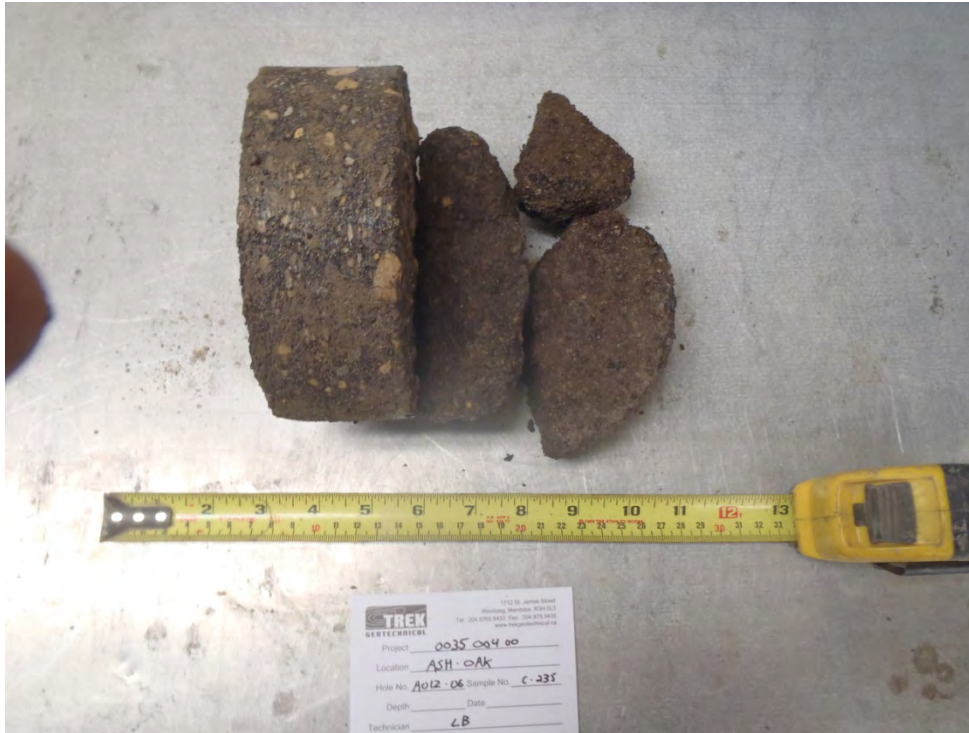
Photo 32: Asphalt core sample from Test Hole AO12-06
