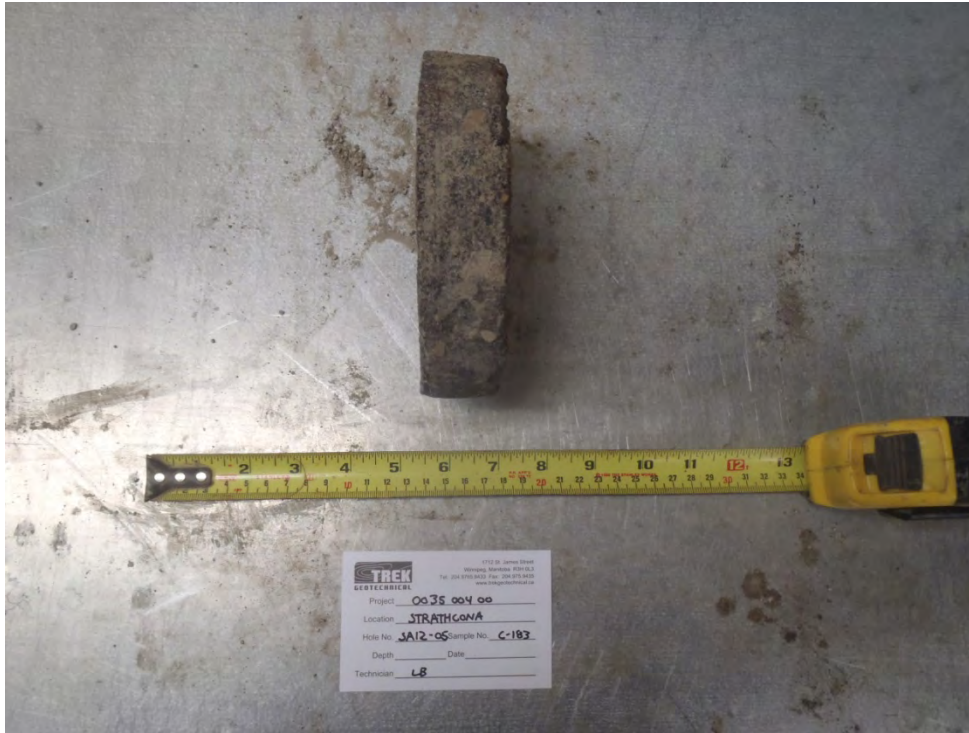
Photo 22: Asphalt core sample from Test Hole SA12-05
