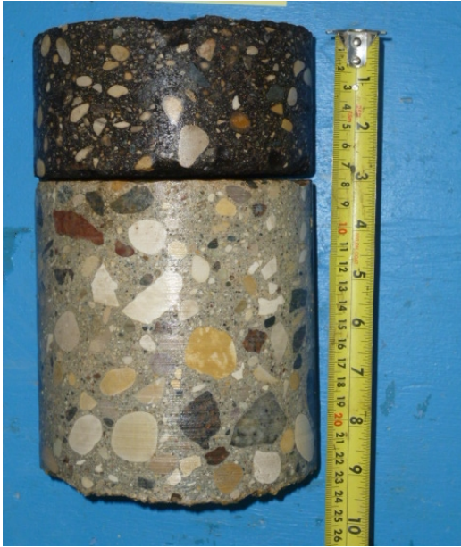
Core Sample from Testhole TH5
