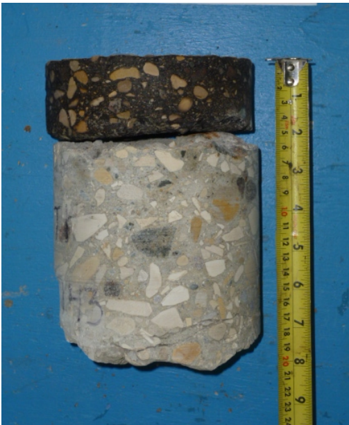
Core Sample from Testhole TH3
