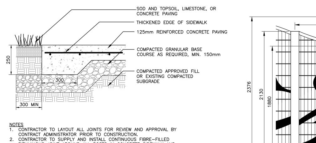
BITUMINOUS JOINT AROUND ALL POSTS IN CONCRETE SIDEWALK AND CONCRETE FOUNDATIONS JOINTS AS PER CITY OF WINNIPEG SPECIFICATIONS.
