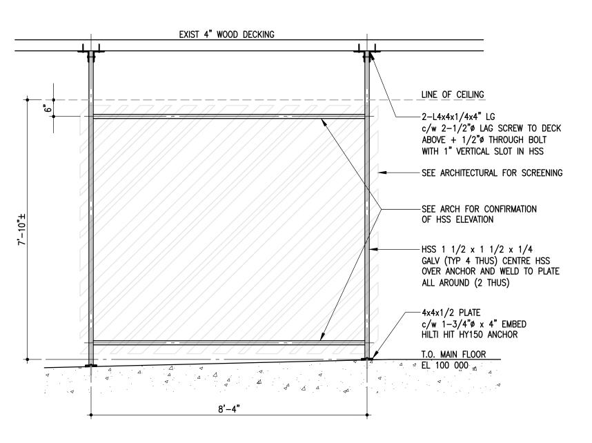
METAL SCREEN ELEVATION DETAIL S-2 | SCALE: 1/2" = 1'-0"
