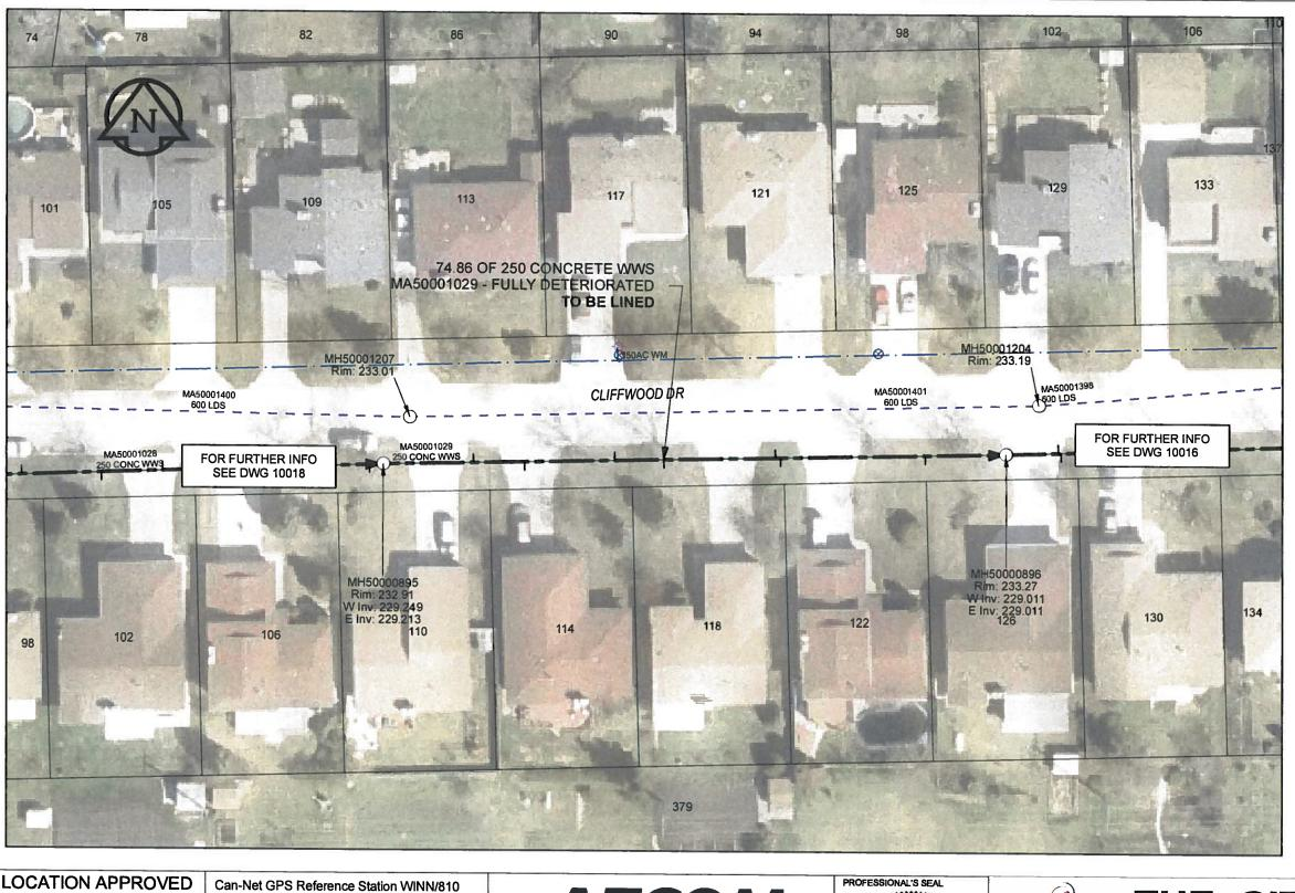
**SEWER JUNCTION INFORMATION** DIST FROM\* **REF MH** SIZE\* CLOCK AT\* MH50000895 10.90 100Ø MH50000895 17.00 100Ø 03 MH50000895 27.80 100Ø 09 MH50000895 33.70 100Ø 02 MH50000895 47.10
