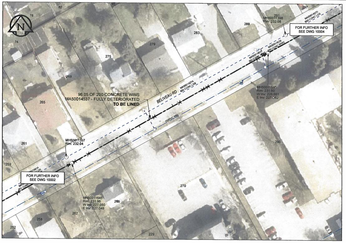
**SEWER JUNCTION INFORMATION REF MH\*** FROM **REF MH** SIZE\* **CLOCK AT\*** MH50011645 150Ø 12 MH50011645 3.80 150Ø 01 MH50011645 8.10 150Ø 12 MH50011645 28.10 150Ø 12 MH50011645 32.90 150Ø 01 MH50011645 40.40 150Ø 12 MH50011645 150Ø 11 MH50011645 52.70 150Ø MH50011645 64.30 150Ø 12 MH50011645 66.50 150Ø 12 MH50011645 72.60 150Ø 12 MH50011645 90.90 150Ø 12 MH50011645 93.30 150Ø \*JUNCTION INFORMATION FROM VIDEO INSPECTION
