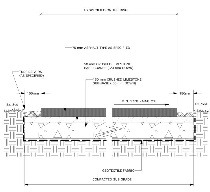
ASPHALT PATHWAY CROSS SECTION
