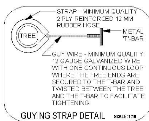
GUYING STRAP DETAIL SCALE 1:10
