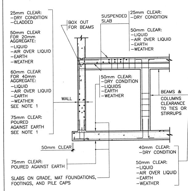
1. PROVIDE 50mm CLEARANCE ON FACE EXPOSED TO DRY CONDITION.
