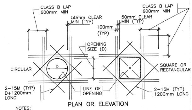
1. FOR OPENINGS D=400mm OR LARGER: ADD EXTRA BARS ON EACH SIDE OF THE OPENING, EQUIVALENT TO HALF THE TOTAL AREA OF REINFORCING CUT IN EACH DIRECTION, EACH FACE, UNLESS NOTED OTHERWISE.
