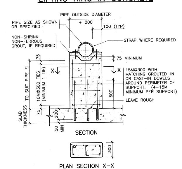
TYPICAL CONCRETE PIPE SUPPORT
