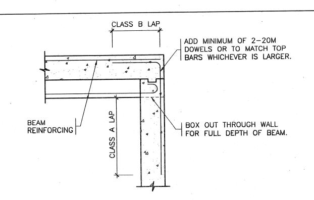
CONCRETE BEAM END REINFORCING
