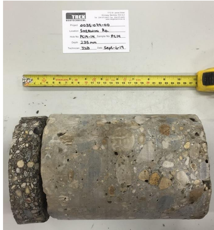
Photo 14: Pavement Core Sample at Test Hole TH19-14
