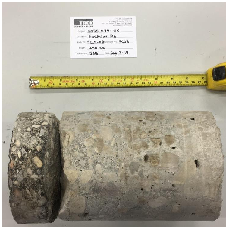
Photo 8: Pavement Core Sample at Test Hole TH19-08
