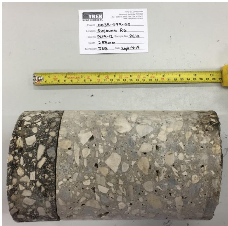
Photo 12: Pavement Core Sample at Test Hole TH19-12
