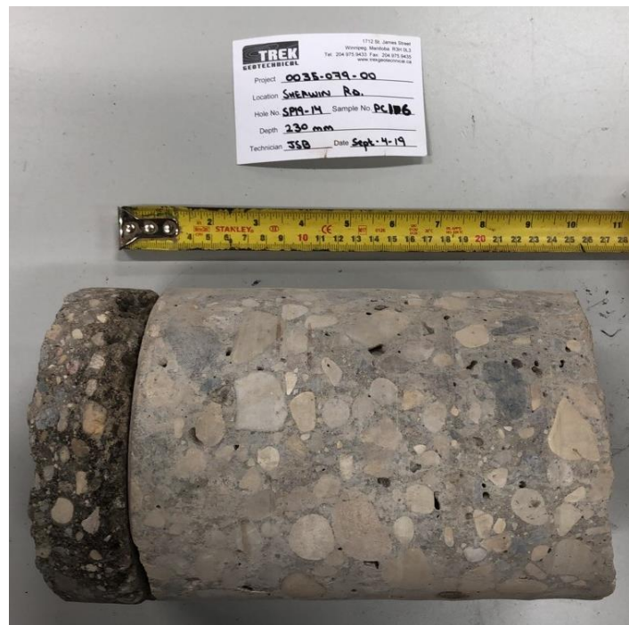
Photo 16: Pavement Core Sample at Test Hole SP19-14
