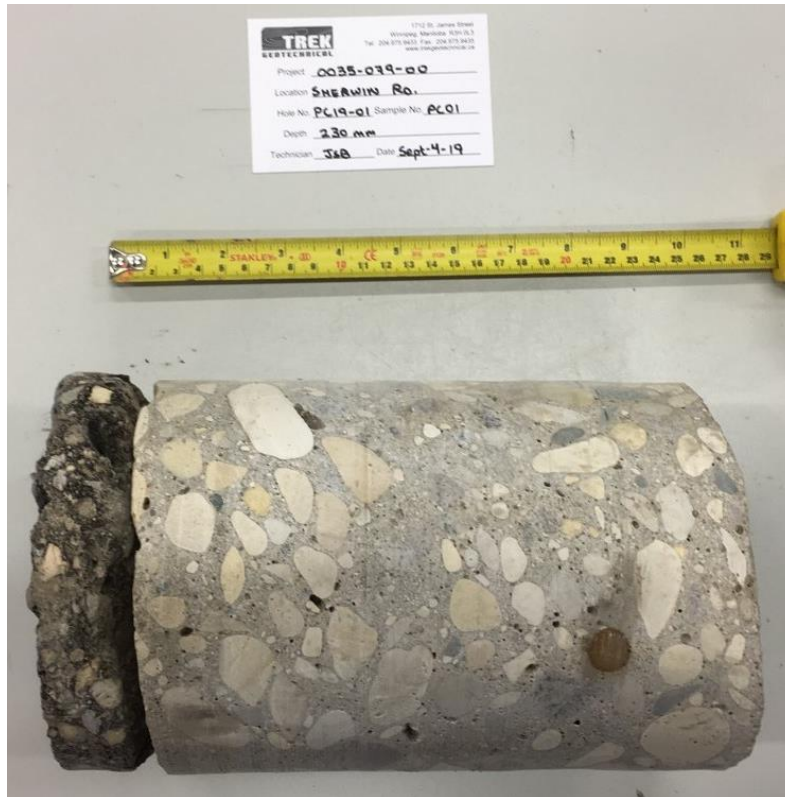
Photo 1: Pavement Core Sample at Test Hole TH19-01
