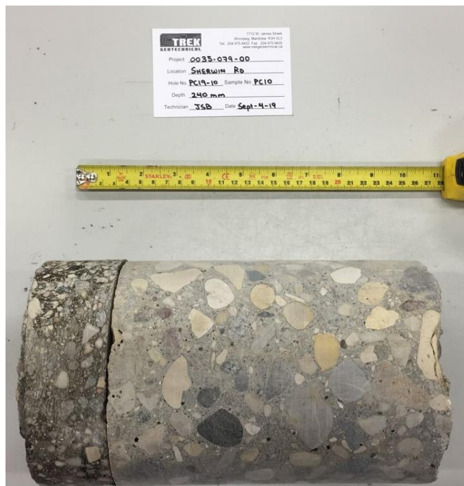
Photo 10: Pavement Core Sample at Test Hole TH19-10
