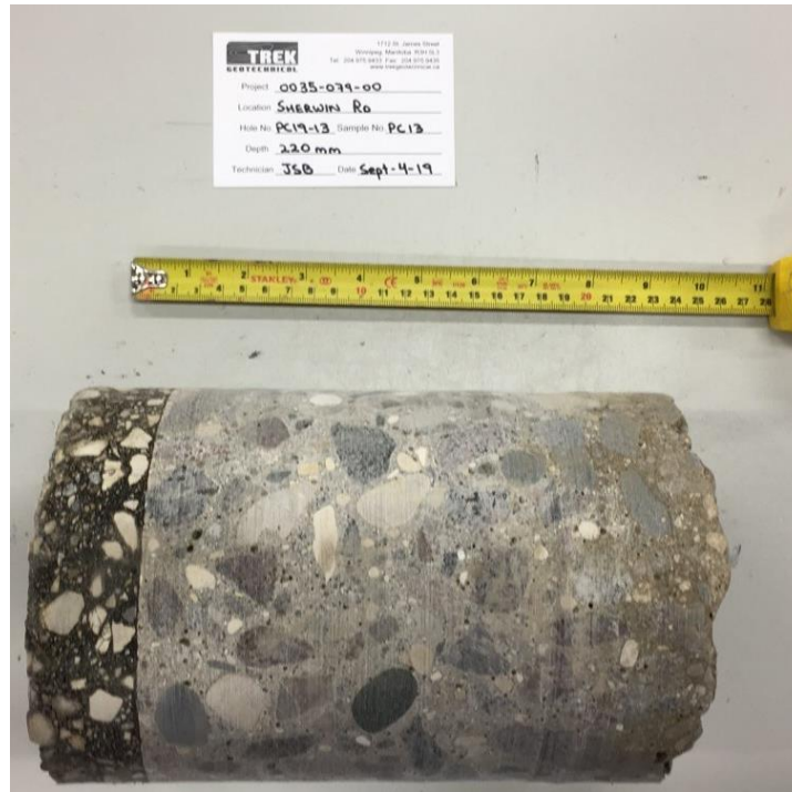
Photo 13: Pavement Core Sample at Test Hole TH19-13
