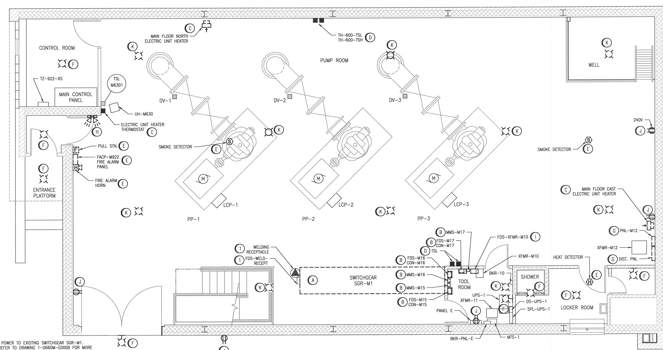
DEMOLISH INCOMING UTILITY POWER SERVICE POWER TO EXISTING SWITCHGEAR SGR-M1. DEMOLISH AND REMOVE EXISTING SGR-M1. REFER TO DRAWING 1-0660M-E0006 FOR MORE
