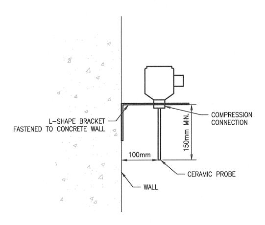
TEMPERATURE TRANSMITTER - WALL MOUNT SCALE: NTS
