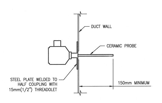
TEMPERATURE TRANSMITTER - UN-INSULATED DUCT SCALE: NTS
