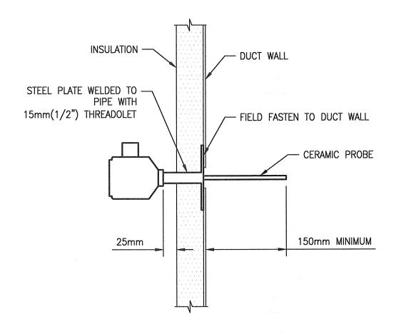
TEMPERATURE TRANSMITTER - INSULATED DUCT SCALE: NTS
