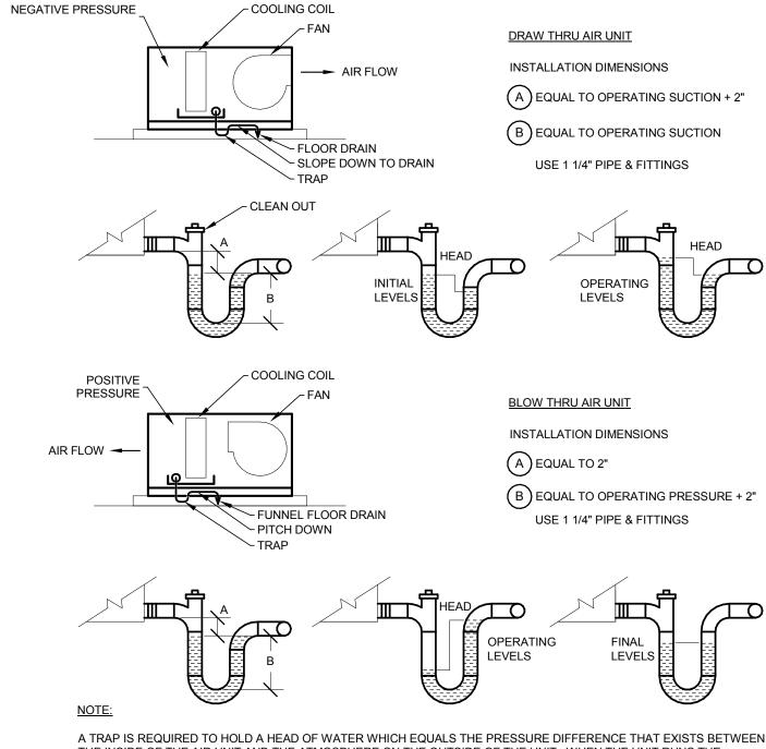
A TRAP IS REQUIRED TO HOLD A HEAD OF WATER WHICH EQUALS THE PRESSURE DIFFERENCE THAT EXISTS BETWEEN THE INSIDE OF THE AIR UNIT AND THE ATMOSPHERE ON THE OUTSIDE OF THE UNIT. WHEN THE UNIT RUNS THE DIFFERENTIAL PRESSURE CAUSES THE WATER IN THE TRAP TO MOVE VERTICALLY. THIS PRODUCES A WATER COLUMN OF SUFFICIENT HEIGHT TO BALANCE THE PRESSURE DIFFERENCE. ONCE THE WATER COLUMN IS ESTABLISHED, ADDITIONAL CONDENSATE SIMPLY FILLS AND OVERFLOWS THE TRAP ON ITS WAY TO THE DRAIN.
