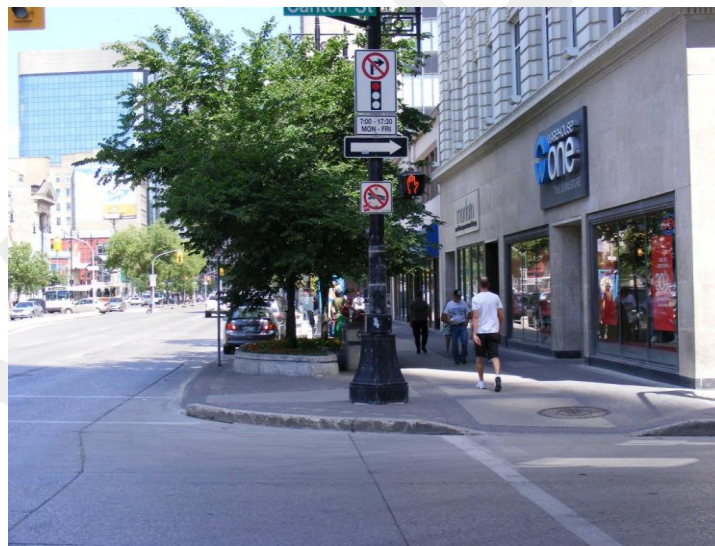
Figure 4.15 – Bump-outs on Portage Avenue allow for more landscaping and reduce the pedestrian crossing distances
