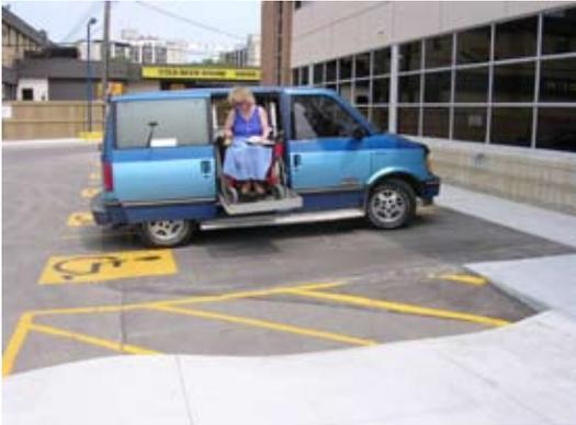
Accessible parking should be wide enough for side-loading vehicles and deep enough for rear loading vehicles.
