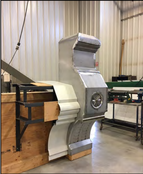
Fabrication of metal corner, Metal Tech Industries, Winnipeg
