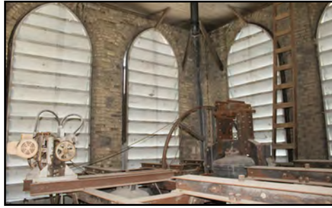
Clock mechanism in the tower of St. Luke's Anglican Church, 130 Nassau Street North
