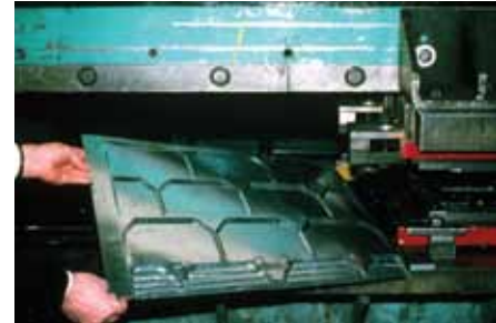
A surviving pressed metal shingle was used as a prototype for manufacturing replacement shingles when restoring the main house at the Motherwell Homestead near Abernathy, SK. In Restoration, repairs or replacements of extensively deteriorated or missing parts of features are done in kind, and are based on physical, documentary and oral evidence.
