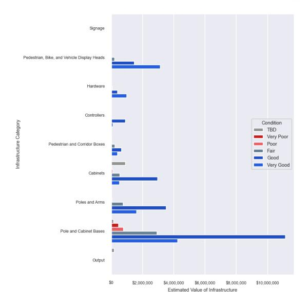
Figure 31: Total estimated value of infrastructure, by infrastructure type and condition, 2019
