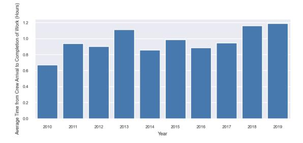
Figure 10: Average time from traffic signal emergency crew arrival to malfunction resolution, by year (2010-2019)
