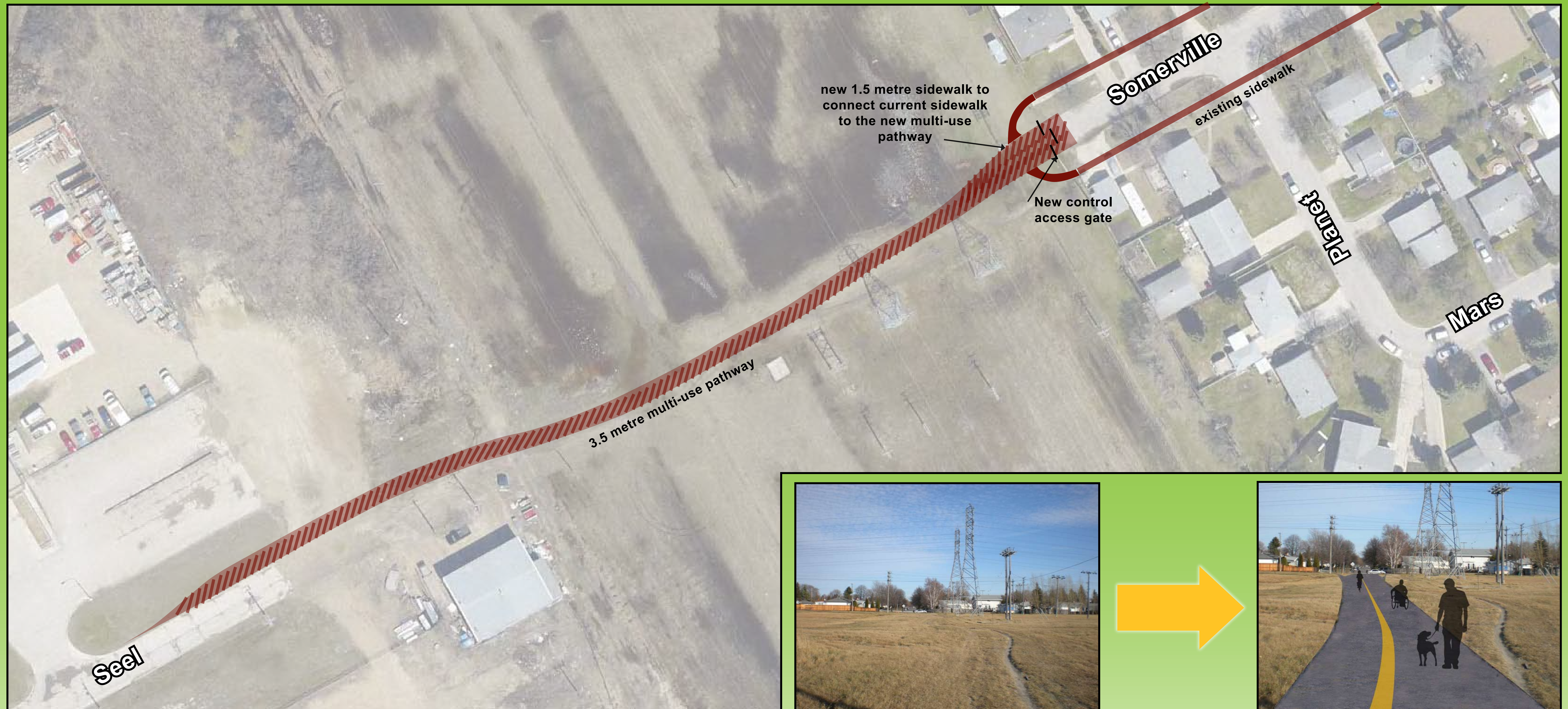
Proposed 3.5 m asphalt multi-use pathway to connect Seel Avenue to Somerville
