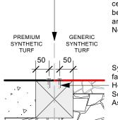
**SYNTHETIC TURFS CONNECTION DETAIL**  Synthetic turfs to meet at centre line of timbers between concrete pitch and granular run ups. No gaps
