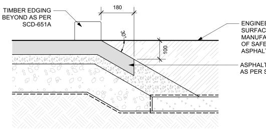
**ENGINEERED WOOD FIBRE SAFETY** SURFACE ON DRAINAGE LAYER AS PER MANUFACTURER'S SPECIFICATIONS. TOP OF SAFETY SURFACING TO BE FLUSH WITH ASPHALT AT ENTRANCE.
