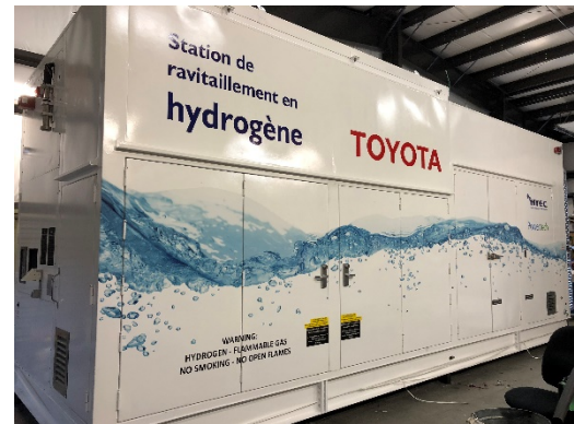
700 Bar T40 Containerized Station
