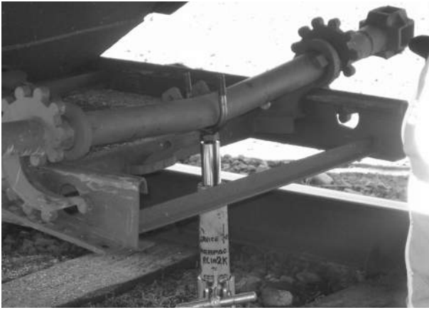
Bent hopper gate being repaired
