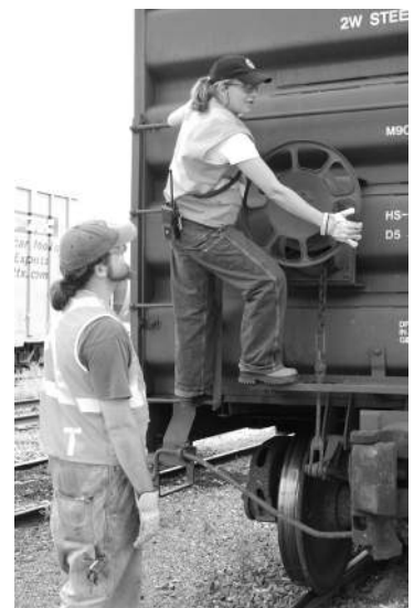
3-point Contact for applying a vertical handbrake
