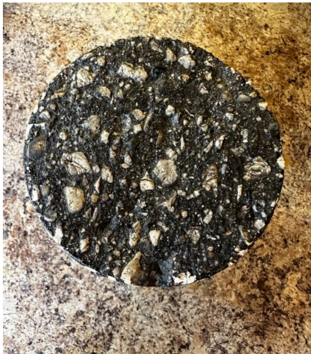
Image 2.2 Core Sample 2 showing Top Surface
