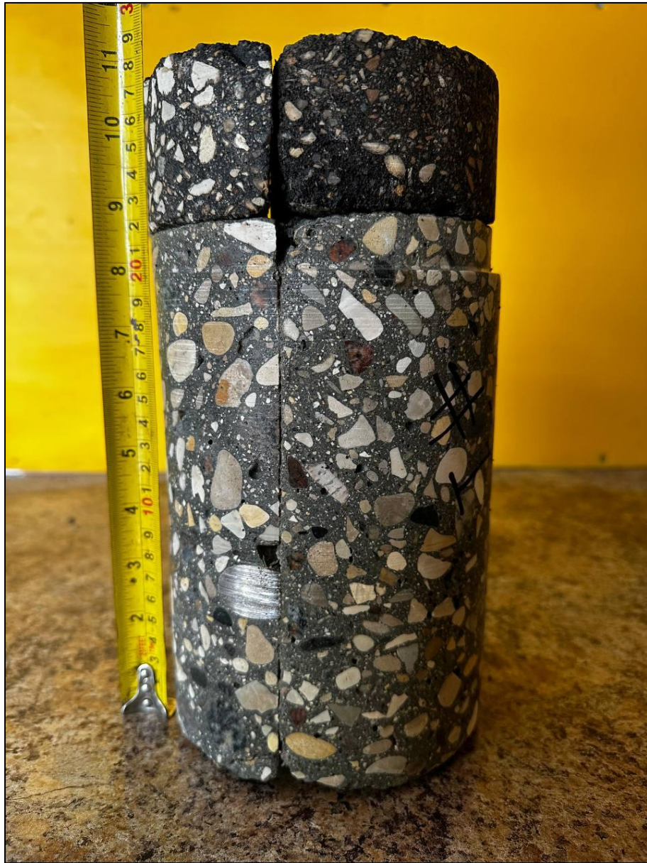
Image 1.1 Core Sample 1 showing measurements
