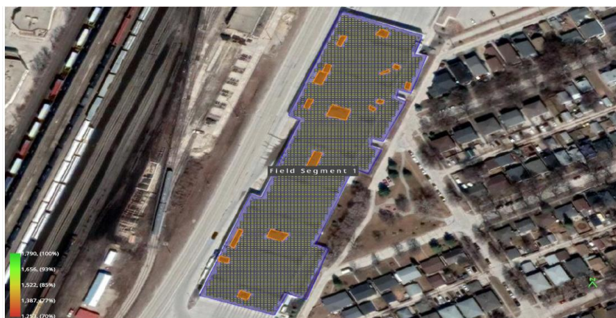
Figure 22: Potential Rooftop Solar Layout
