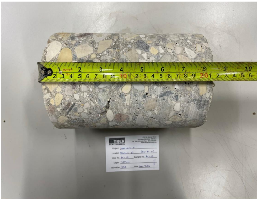
Photo 2: Pavement Core Sample PC-19
