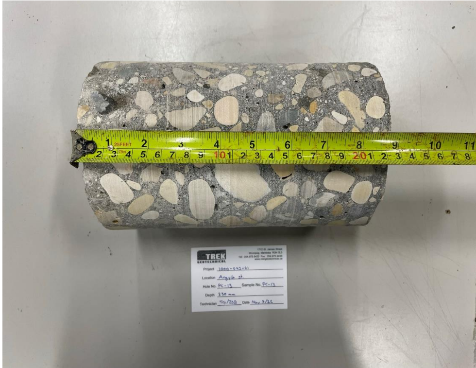
Photo 1: Pavement Core Sample PC-13
