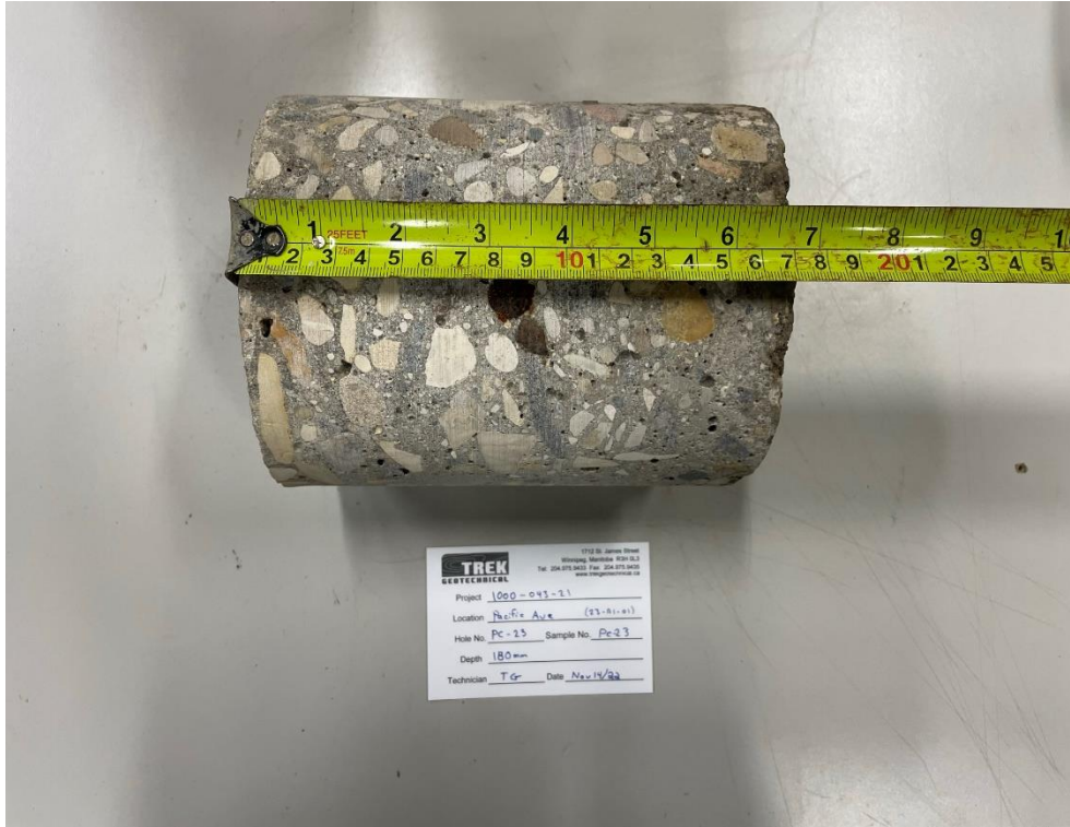
Photo 1: Pavement Core Sample PC-23
