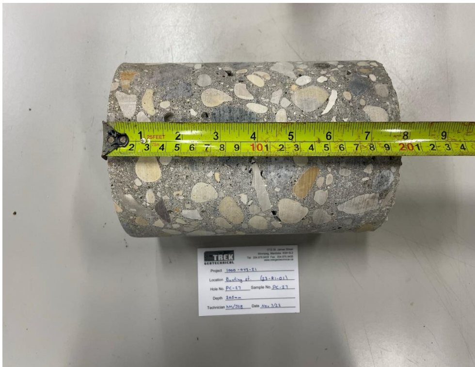
Photo 2: Pavement Core Sample PC-27
