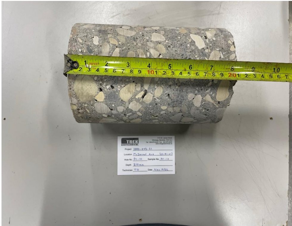
Photo 1: Pavement Core Sample PC-10
