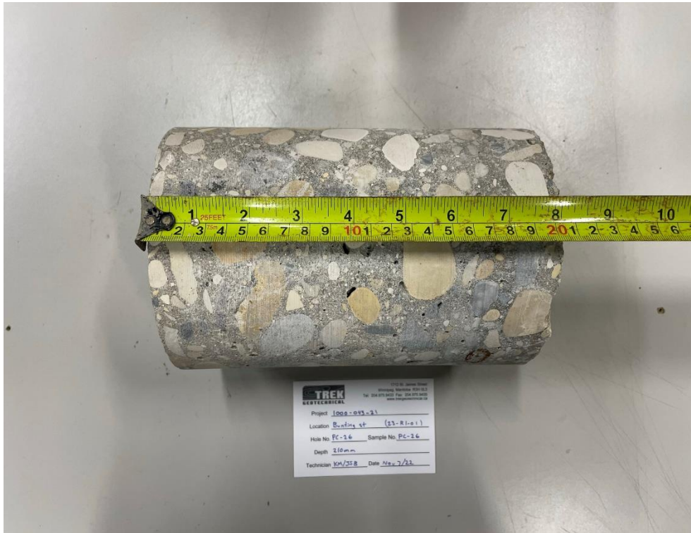
Photo 1: Pavement Core Sample PC-26
