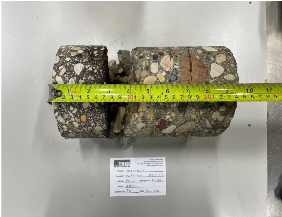
Photo 2: Pavement Core Sample PC-24
