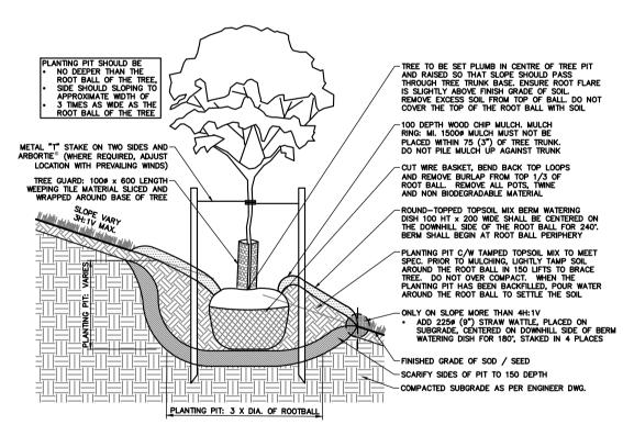
TYPICAL TREE PLANTING ON SLOPE SECTION SCALE: N.T.S.
