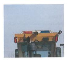
Motor Grader with Dual Rotating Strobe lights, where blue is active <u>only</u> during Winter snow removal
