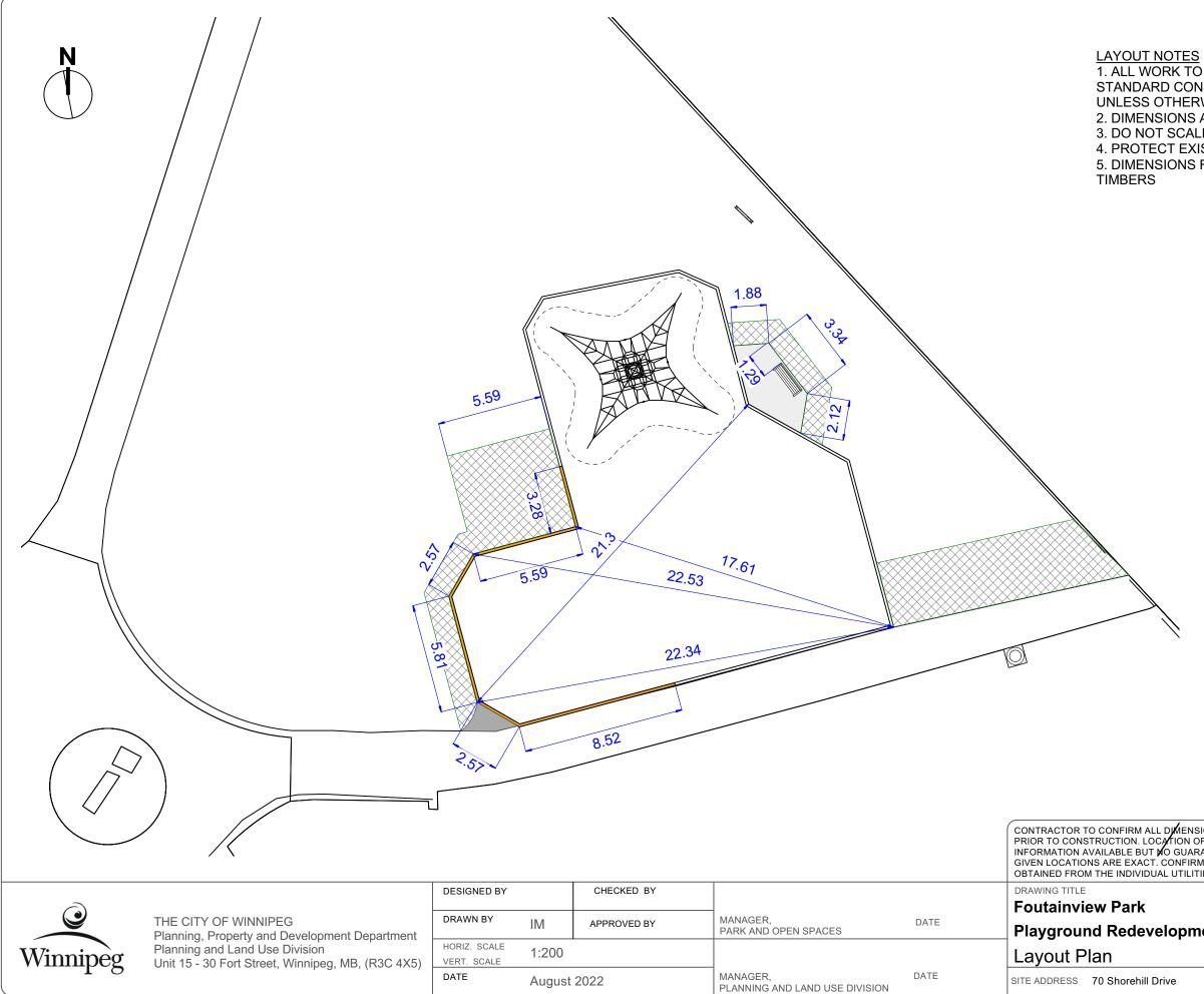
1. ALL WORK TO CONFORM TO CURRENT CITY OF WINNIPEG STANDARD CONSTRUCTION SPECIFICATIONS AND DETAILS UNLESS OTHERWISE NOTED. 2. DIMENSIONS ARE IN METERS UNLESS OTHERWISE NOTED.
