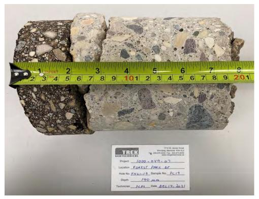
Photo 1: Pavement Core Sample at PC21-19
