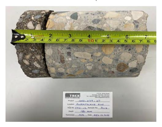
Photo 4: Pavement Core Sample at PC21-12
