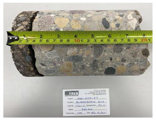
Photo 3: Pavement Core Sample at PC21-11
