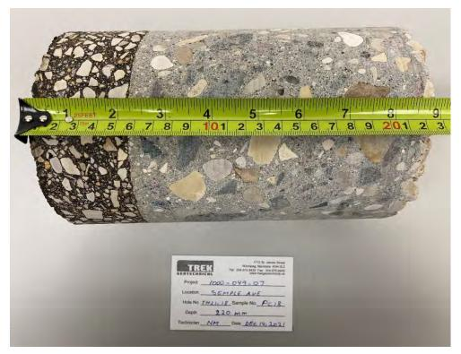
Photo 3: Pavement Core Sample at PC21-18
