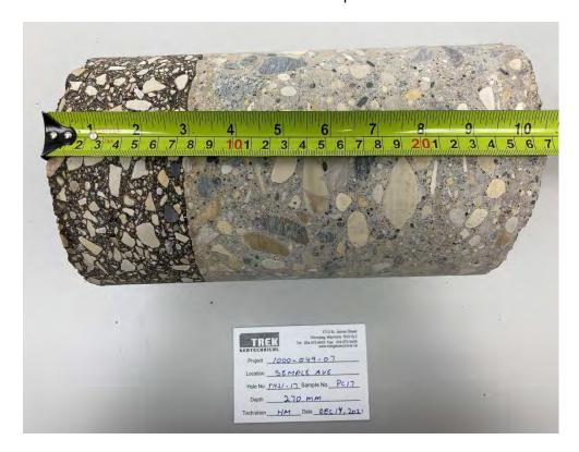
Photo 2: Pavement Core Sample at PC21-17
