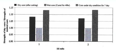
Effect of core moisture condition on core strength for different aspect ratios (l/d).
