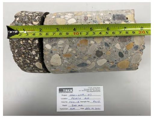
Photo 1: Pavement Core Sample at PC21-13
