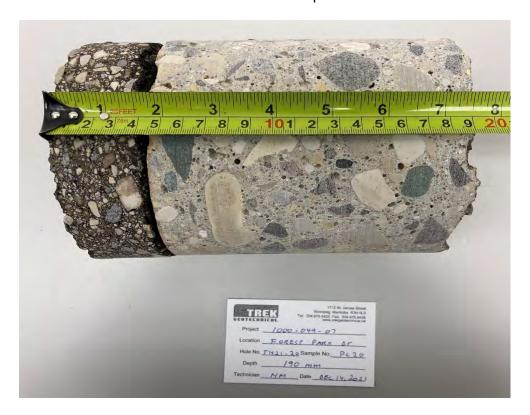
Photo 2: Pavement Core Sample at PC21-20
