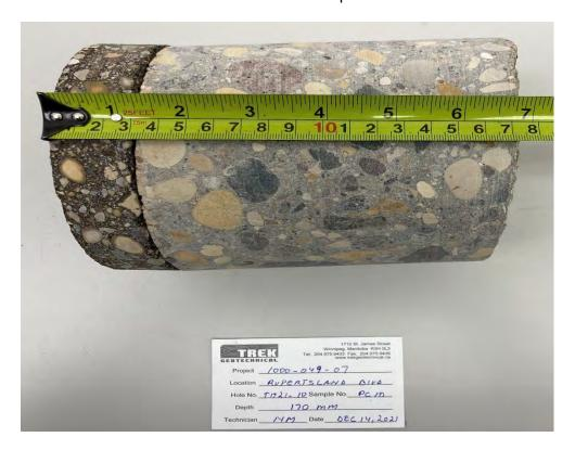
Photo 2: Pavement Core Sample at PC21-10
