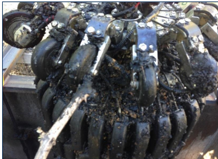
Figure 5: Debris accumulation on 20-inch Chimera tool.
