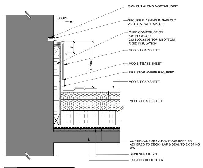
Flashing Detail A1.5 Scale: 1 1/2" = 1'-0"
