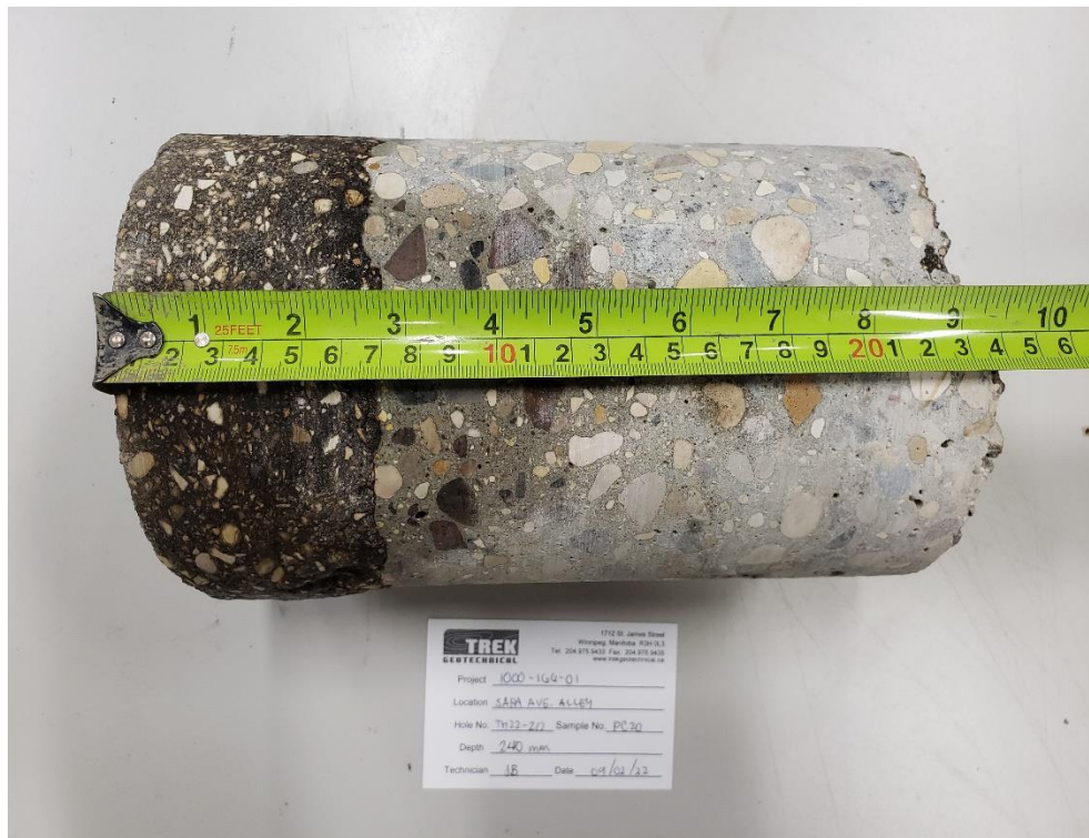
Photo 2: Pavement Core Sample at Test Hole TH22-20
