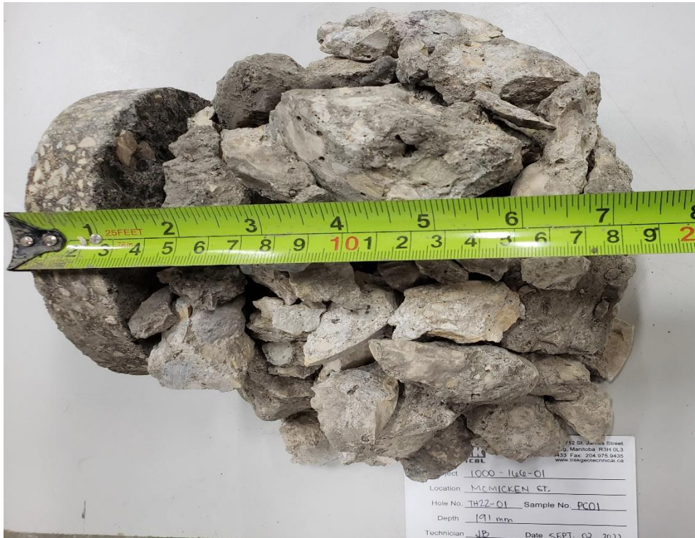
Photo 1: Pavement Core Sample at Test Hole TH22-01
