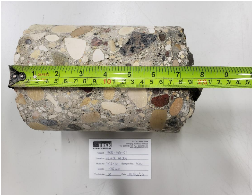
Photo 1: Pavement Core Sample at Test Hole TH22-16
