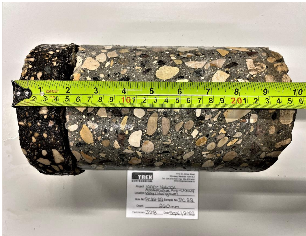
Photo 2: Pavement Core Sample PC-22
