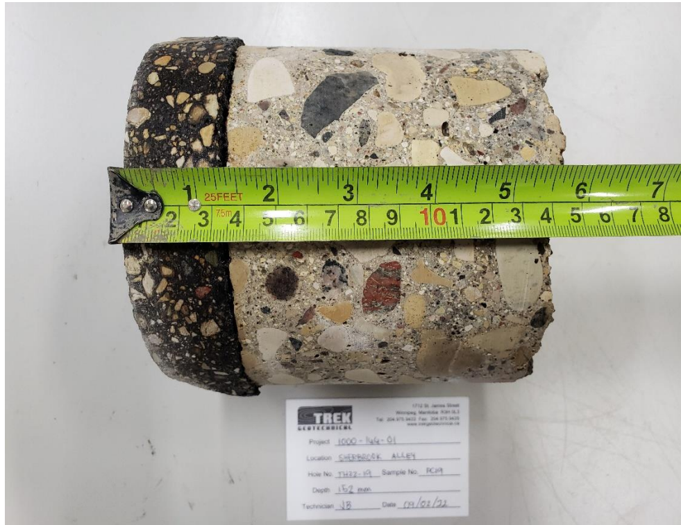
Photo 1: Pavement Core Sample at Test Hole TH22-19
