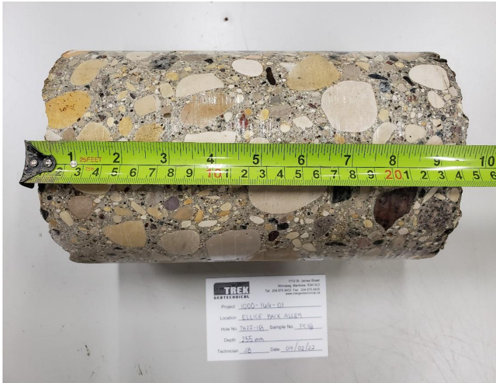
Photo 3: Pavement Core Sample at Test Hole TH22-18
