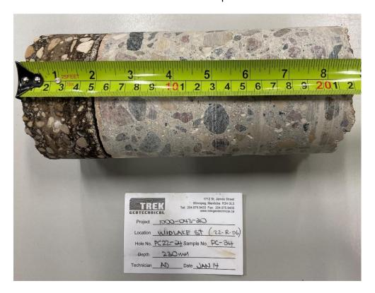
Photo 6: Pavement Core Sample at PC22-24
