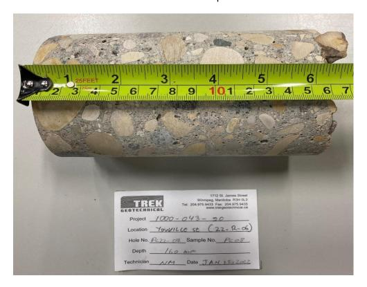
Photo 2: Pavement Core Sample at PC22-08
