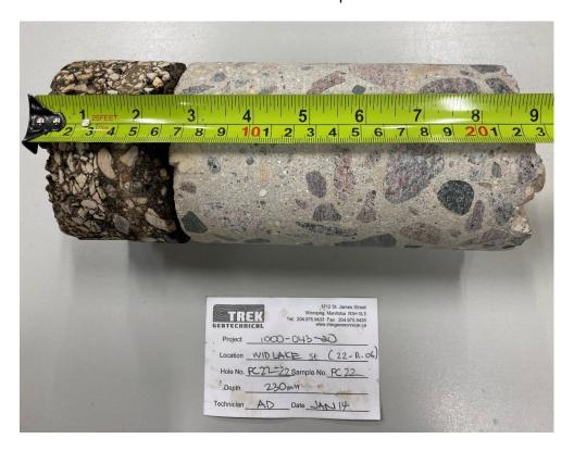
Photo 4: Pavement Core Sample at PC22-22
