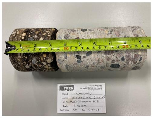
Photo 3: Pavement Core Sample at PC22-21
