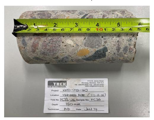
Photo 2: Pavement Core Sample at PC22-26
