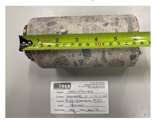
Photo 2: Pavement Core Sample at PC22-20
