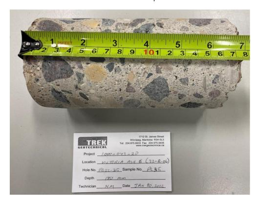
Photo 2: Pavement Core Sample at PC22-35
