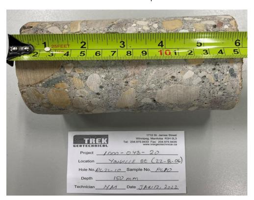
Photo 4: Pavement Core Sample at PC22-10
