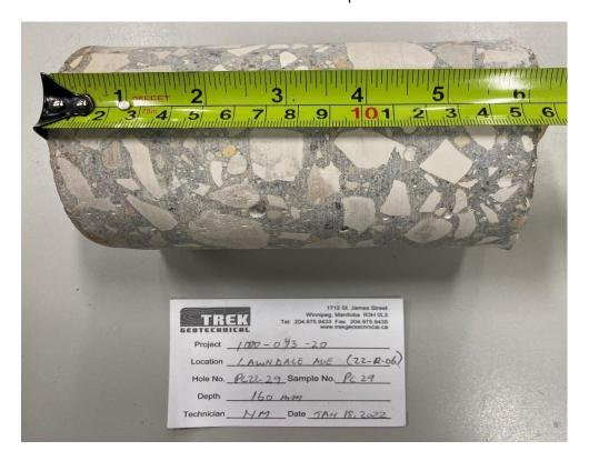
Photo 2: Pavement Core Sample at PC22-29
