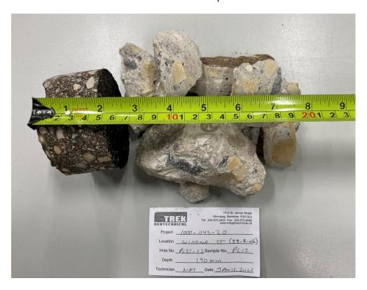
Photo 2: Pavement Core Sample at PC22-12
