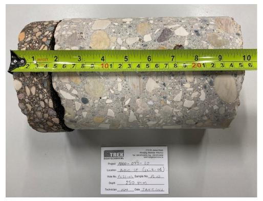
Photo 3: Pavement Core Sample at PC22-03
