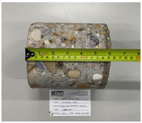
Photo 3: Pavement Core Sample at TH22-03
