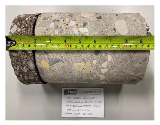
Photo 2: Pavement Core Sample at PC22-02
