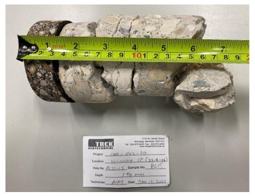
Photo 5: Pavement Core Sample at PC22-15
