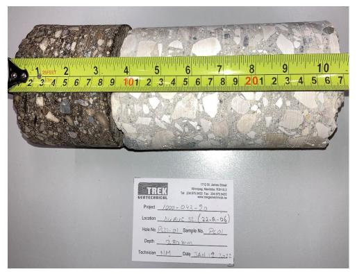
Photo 1: Pavement Core Sample at PC22-01
