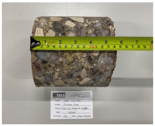
Photo 1: Pavement Core Sample at TH22-01
