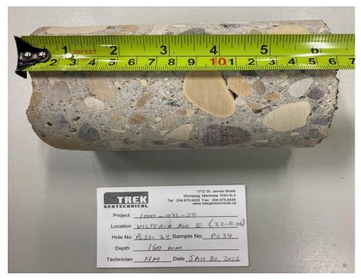
Photo 1: Pavement Core Sample at PC22-34
