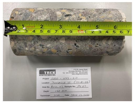
Photo 1: Pavement Core Sample at PC22-07
