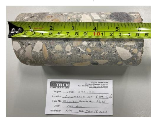
Photo 4: Pavement Core Sample at PC22-31
