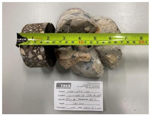
Photo 1: Pavement Core Sample at PC22-11
