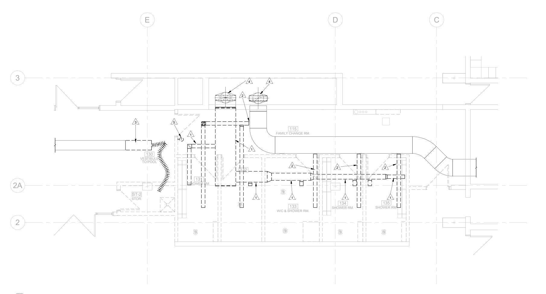
MAIN FLOOR PARTIAL PLAN - HVAC DEMOLITION
