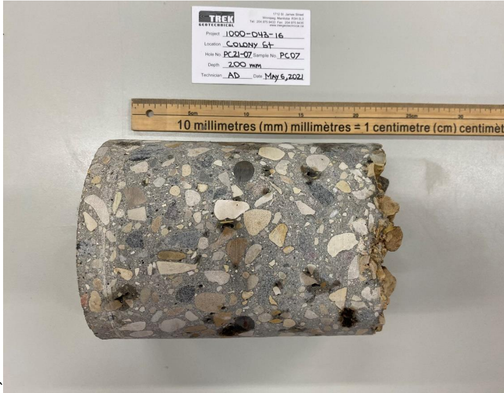
Photo 3: Pavement Core Sample at PC21-07
