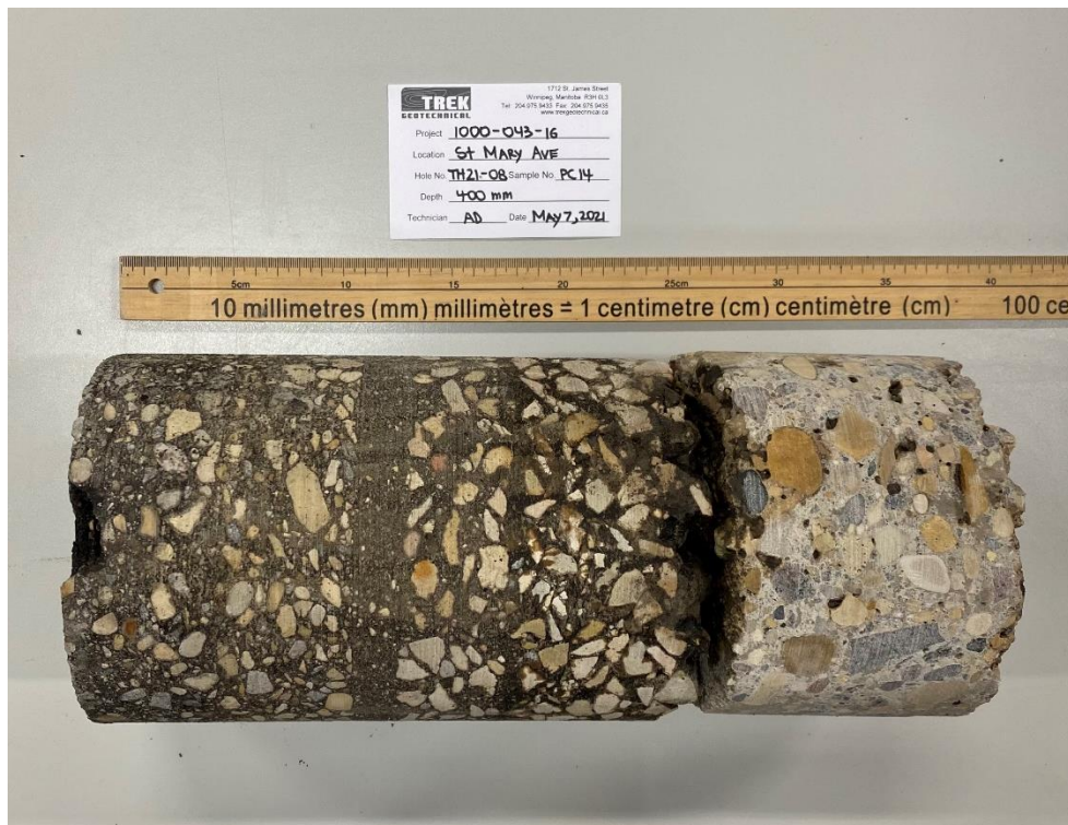
Photo 2: Pavement Core Sample at Test Hole TH21-08
