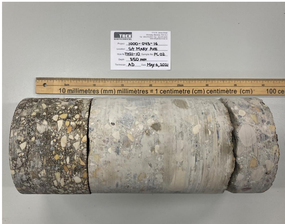
Photo 4: Pavement Core Sample at Test Hole TH21-10
