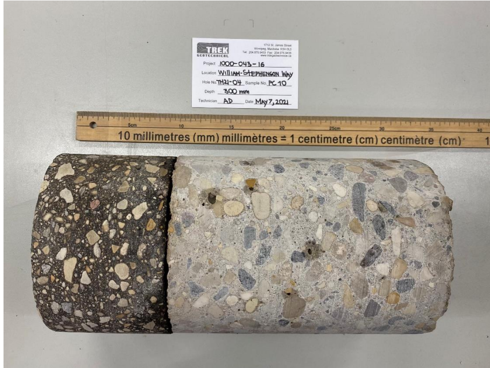
Photo 1: Pavement Core Sample at Test Hole TH21-04
