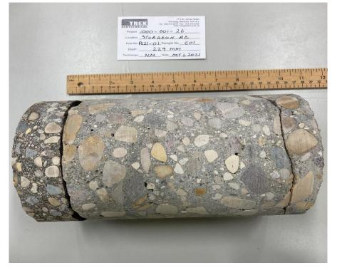
Photo 1: Pavement Core Sample at PC21-01
