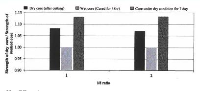
Figure 20 Effect of core moisture condition on core strength for different aspect ratios (l/d).
