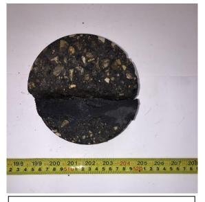
LEO-05: Asphalt Layer, Plan View
