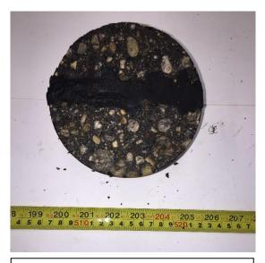
LEO-06: Asphalt Layer, Plan View
