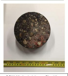
BOW-02: Asphalt Layer, Plan View
