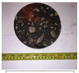
LEO-02: Asphalt Layer, Plan View
