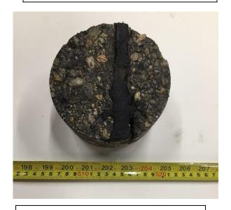
BOW-04: Asphalt Layer, Plan View
